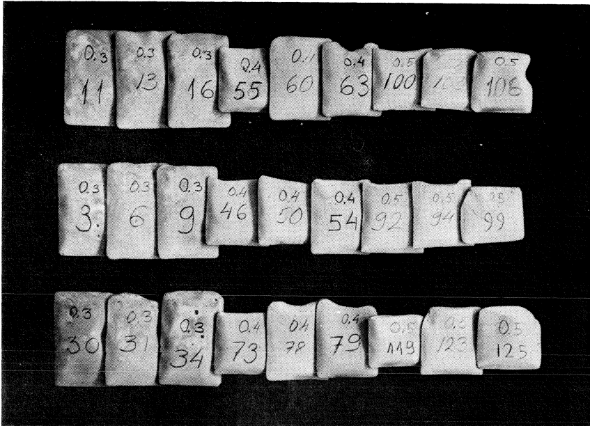
Photo 1. Some cement paste specimens for determination of equilibrium moisture content (sorption isotherms). Water cement ratios 0.3, 0.4, 0.5 are shown. The specimens were poured into plastic bags 6 cm by 9 cm.
