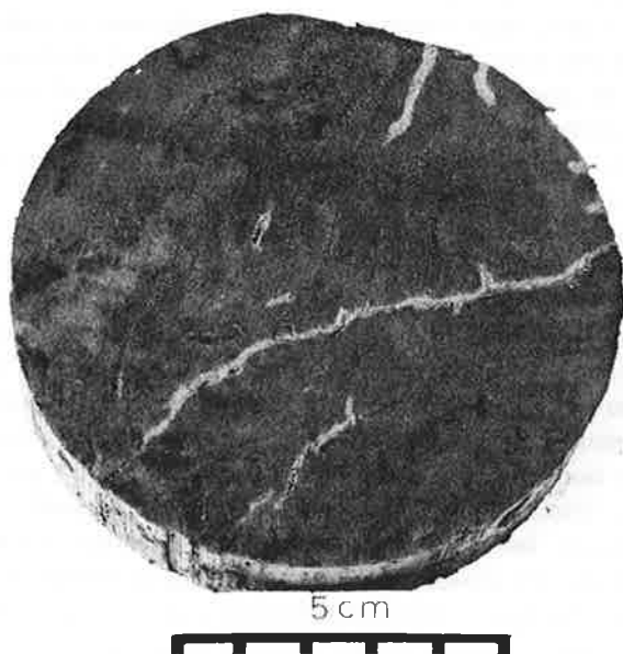
Fig. 3. Oxidized cracks (in situ) in Littorina sediment, Sipoo.
