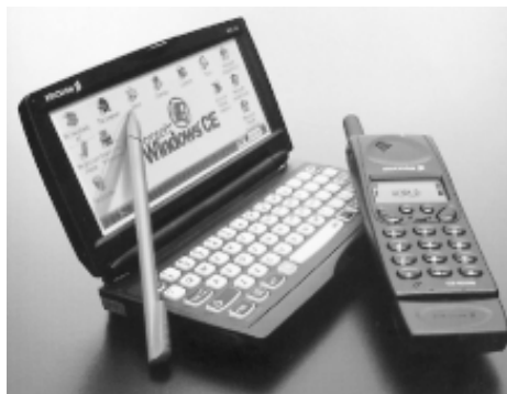
Fig. 5. Ericsson's MC 16 is a combination of a mobile phone and a PDA.
