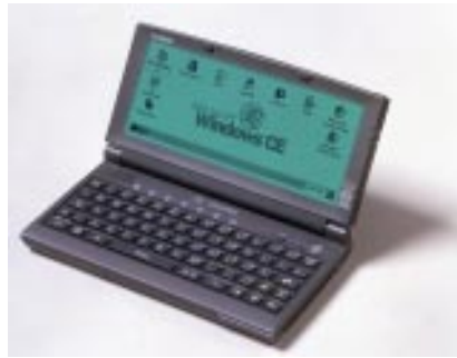
Fig. 3. The keyboard of a hand-held PC is quite small. The screens are touch-sensitive with 16 or 256 colours. A pen can be used like the mouse, or it can be used for writing, if the device has handwriting recognition. Shortcut buttons are applied in hand-held PCs. They may be located in the upper part of the keyboard or sometimes on the screen.
