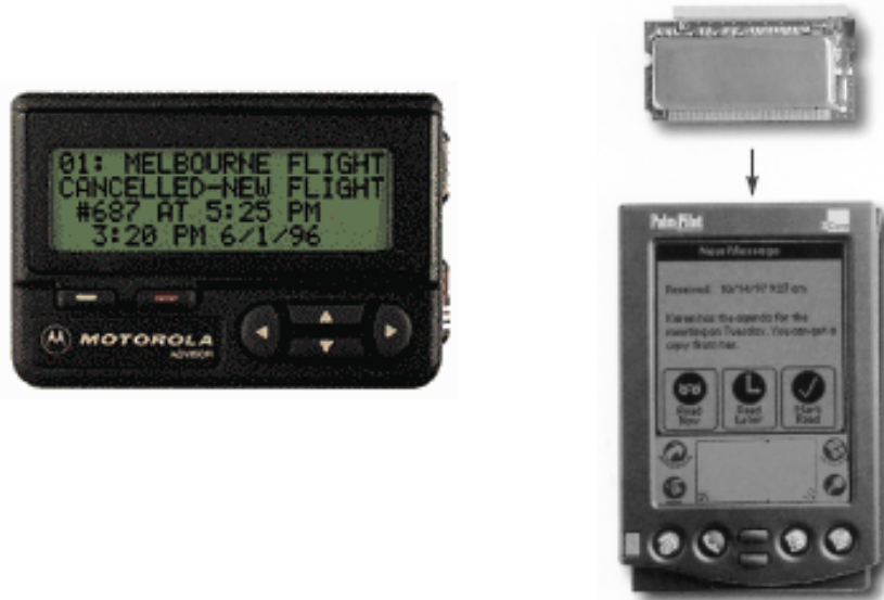
Fig. 6. A pager (left). A PDA device can be turned into a pager using a special plug-in pager card (right).
