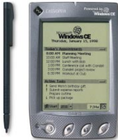
Fig. 3. The keyboard of a hand-held PC is quite small. The screens are touch-sensitive with 16 or 256 colours. A pen can be used like the mouse, or it can be used for writing, if the device has handwriting recognition. Shortcut buttons are applied in hand-held PCs. They may be located in the upper part of the keyboard or sometimes on the screen.
