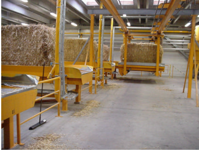
Figure 18. The traversing table has picked up a bale from the right and passes it now on to a vacant feeder line to the left /2/.
