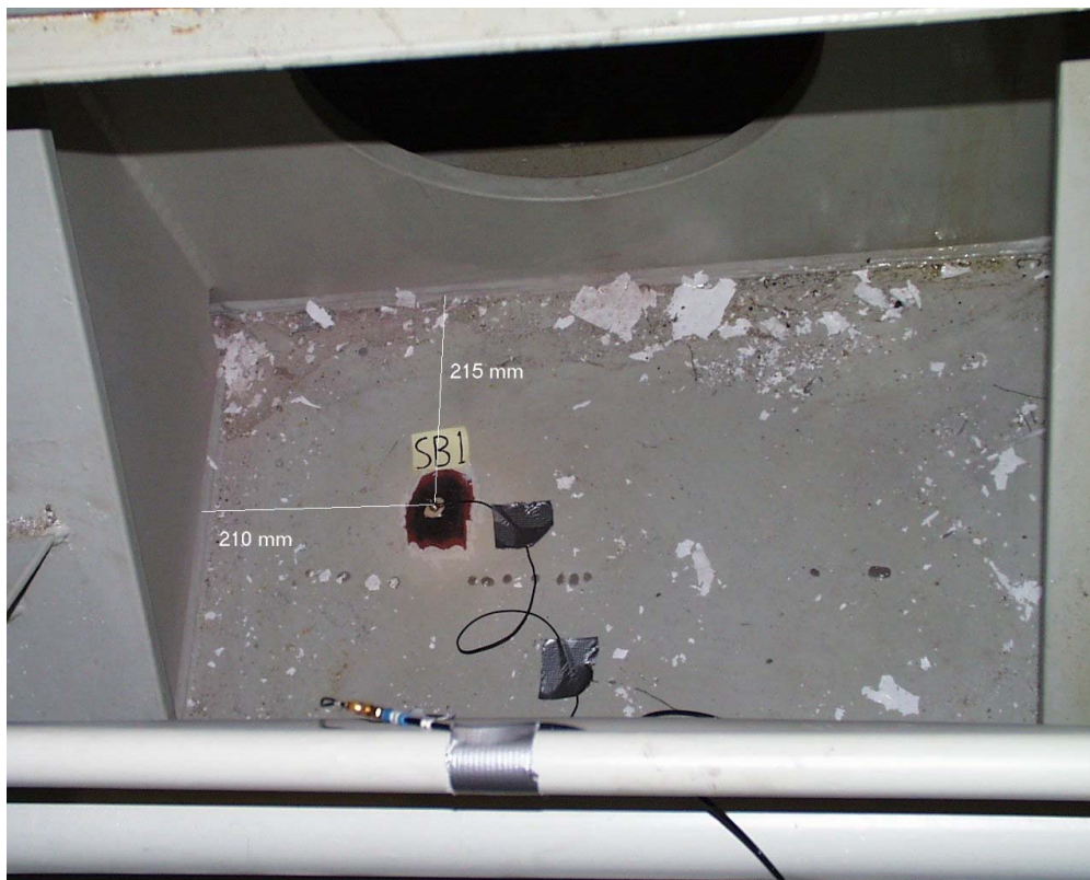
Figure 3. Measuring point SB1; accelerometer glued to the target (mounting base level of the main engine nr.2 is seen at the upper left corner of the photograph).
