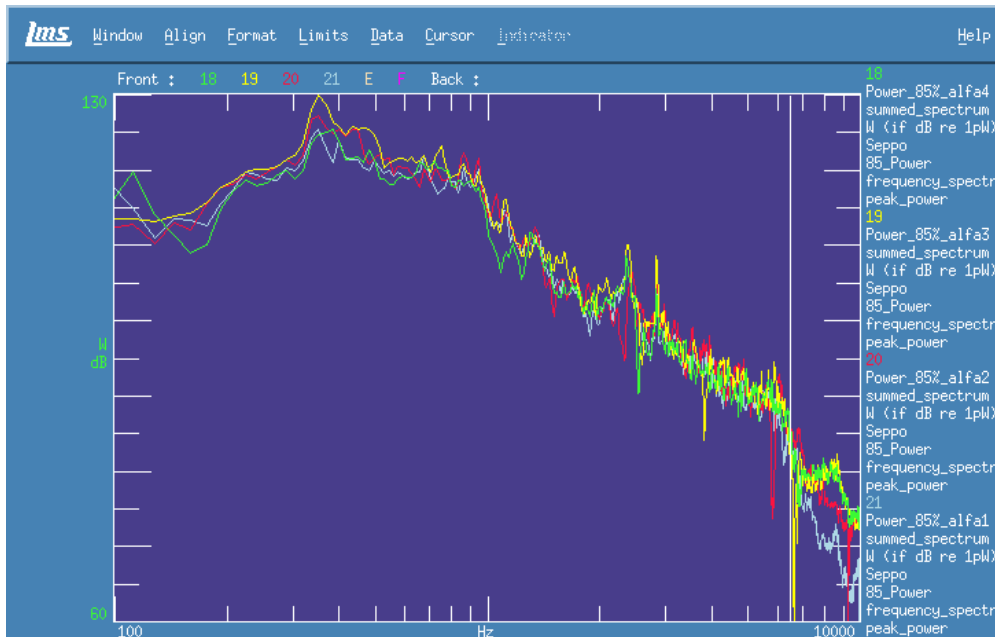
Figure 26. Vibrational power (dB, re 1e-12 W, logarithmic axes) at load of 85% during sea voyage calculated with four different proportionality functions Re(\hat{\alpha}) .
