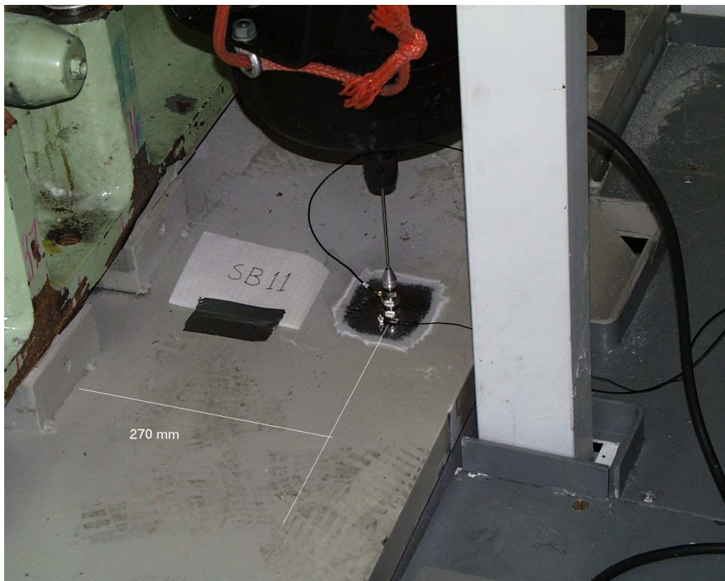
Figure 2. Vertical excitation with electrodynamic shaker (excitation point SB11).
