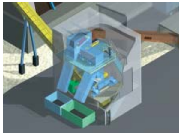
Screening of fuel before combustion. Roxon.
