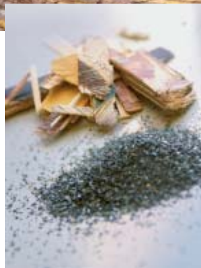
Quartz-free sand enables efficient combustion of alkali-rich fuels such as plywood residue. Kvaerner Power Oy.
