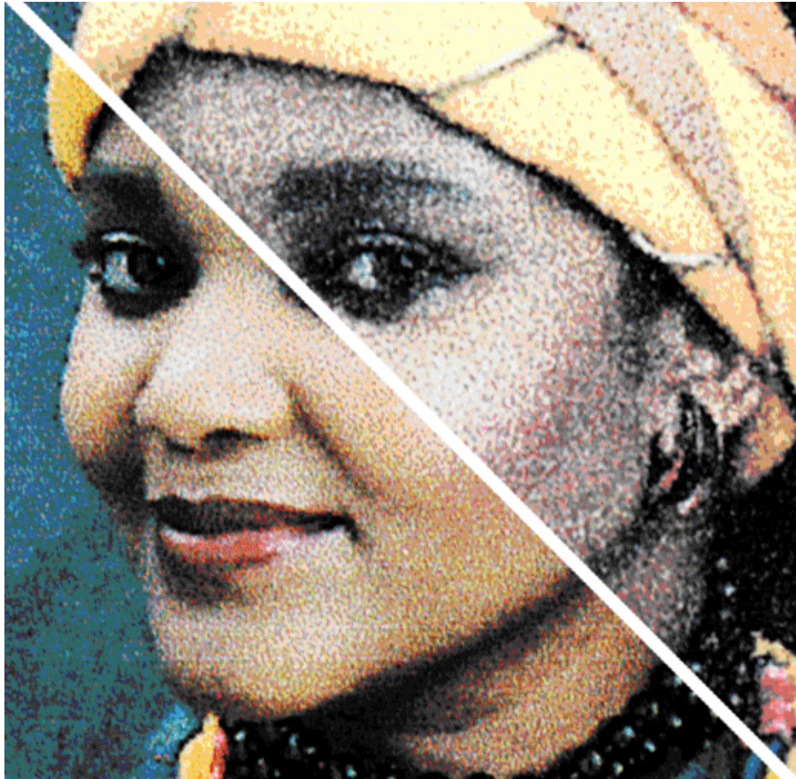
Figure 9. Test picture printed on two coated paper grades printed by the same printer. The print quality in ink jet printing is extremely surface-dependent.
