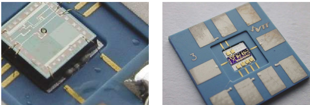
Figure 2. Photo of the PST test component attached on LTCC (left) and a photo of the assembled APH403 MMIC with six capacitors.
