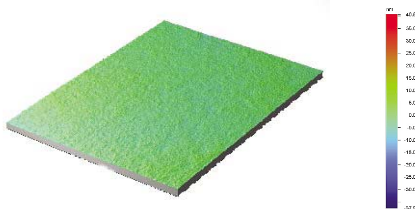
Figure 5. Image of waveguides generated using a White Light Interferometer
