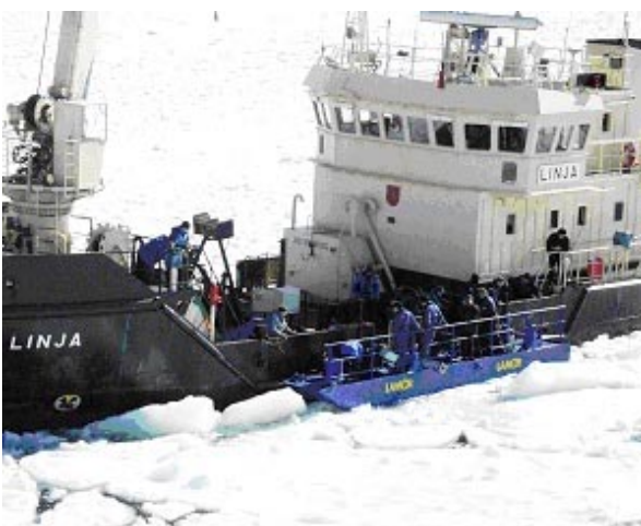
Figure 1. The novel Oil recovery device in the VTT's full-scale trial. This new system has currently mounted onboard oil combating vessel Seili.
