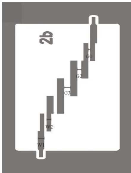
Figure 1. Layout of the designed microstrip band-pass filter.
