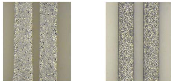
Figure 2. Printed (left) and etched (right) conductors and gap. Designed line and gap widths are 130 and 75 \mu\text{m} , respectively.
