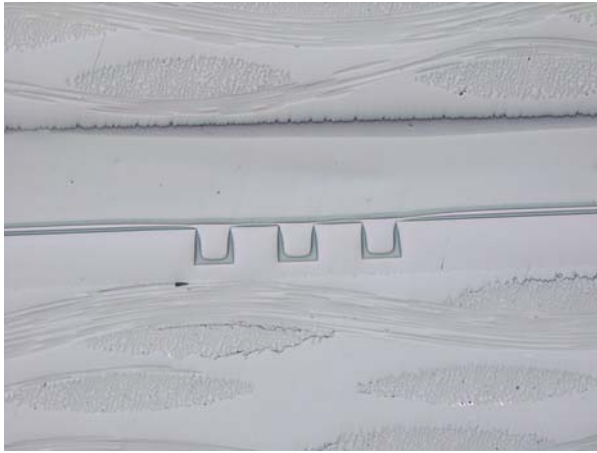
Figure 4: PMMA/SU-8/PMMA waveguides on FR-4 substrate fabricated with two-step groove filling process. After photolithographic waveguide groove structure patterning, 950PMMA is deposited by spinning as under-cladding. SU-8 waveguide cores are then squeegee printed and top-cladded with PMMA cladding layer.
