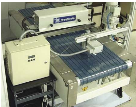
Fig. 2. Developed on-line coating thickness meter on a Barberán curtain coater. Only one sensor head is shown in the picture.
