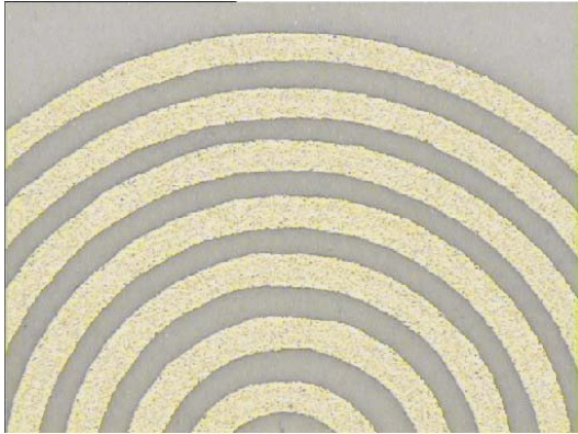
Figure 2. Spiral inductor with line width of 90 \mu\text{m} .
