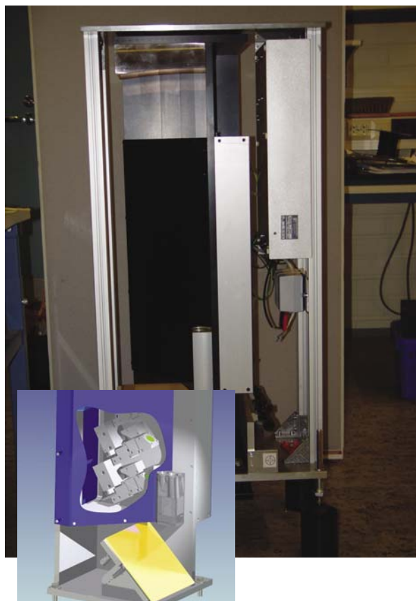
Figure 4. A picture of REVEAL source optics and a 3D CAD model of the optics.
