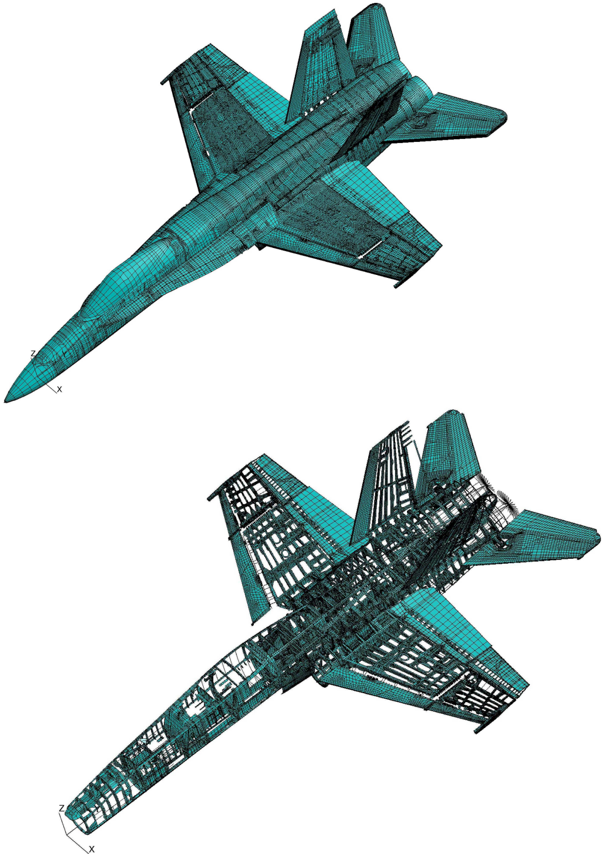
Figure 7. An overview of the Hornet FE model; outer surface (above) and inner structure (below). Courtesy of Patria Aviation, Aircraft Business Unit.
