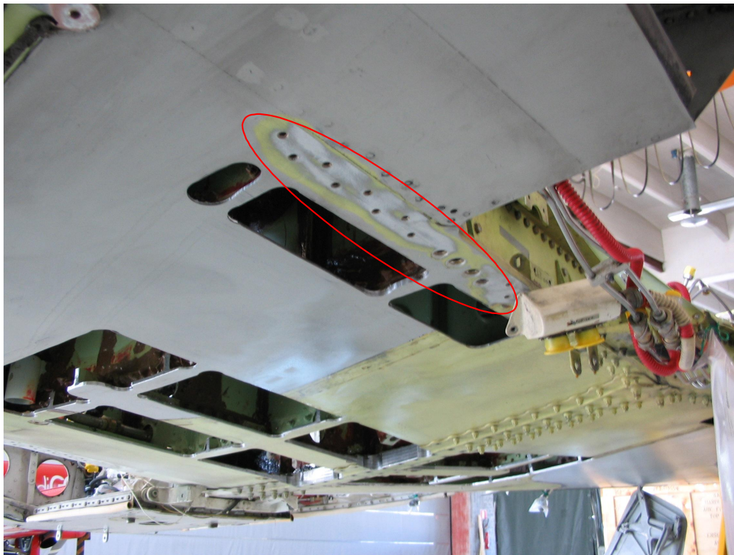
Figure 3 (cont'd). An overview of the FiAF Mk.51 Hawk premod 999 wing teardown inspection: f) Example of holes cut to the lower surface of the wing. Note removed fasteners. Courtesy of Patria Aviation.
