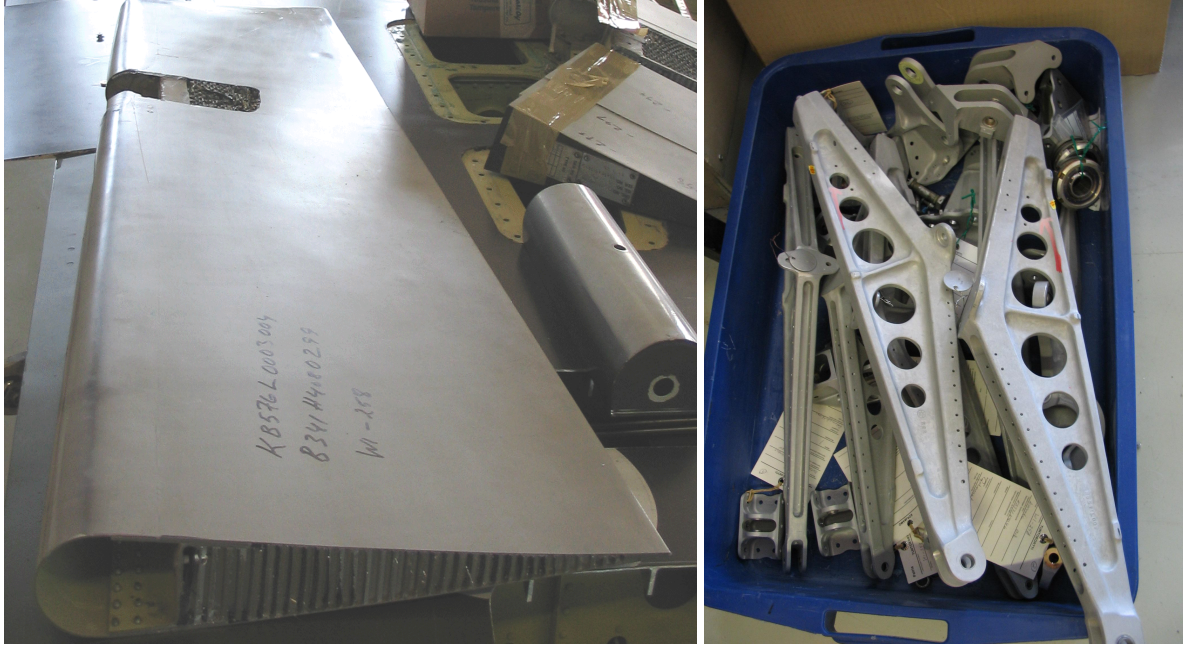
Figure 3. An overview of the FiAF Mk.51 Hawk premod 999 wing teardown inspection: a) an aileron cut for the inspections; b) examples of removed and inspected parts. Courtesy of Patria Aviation.
