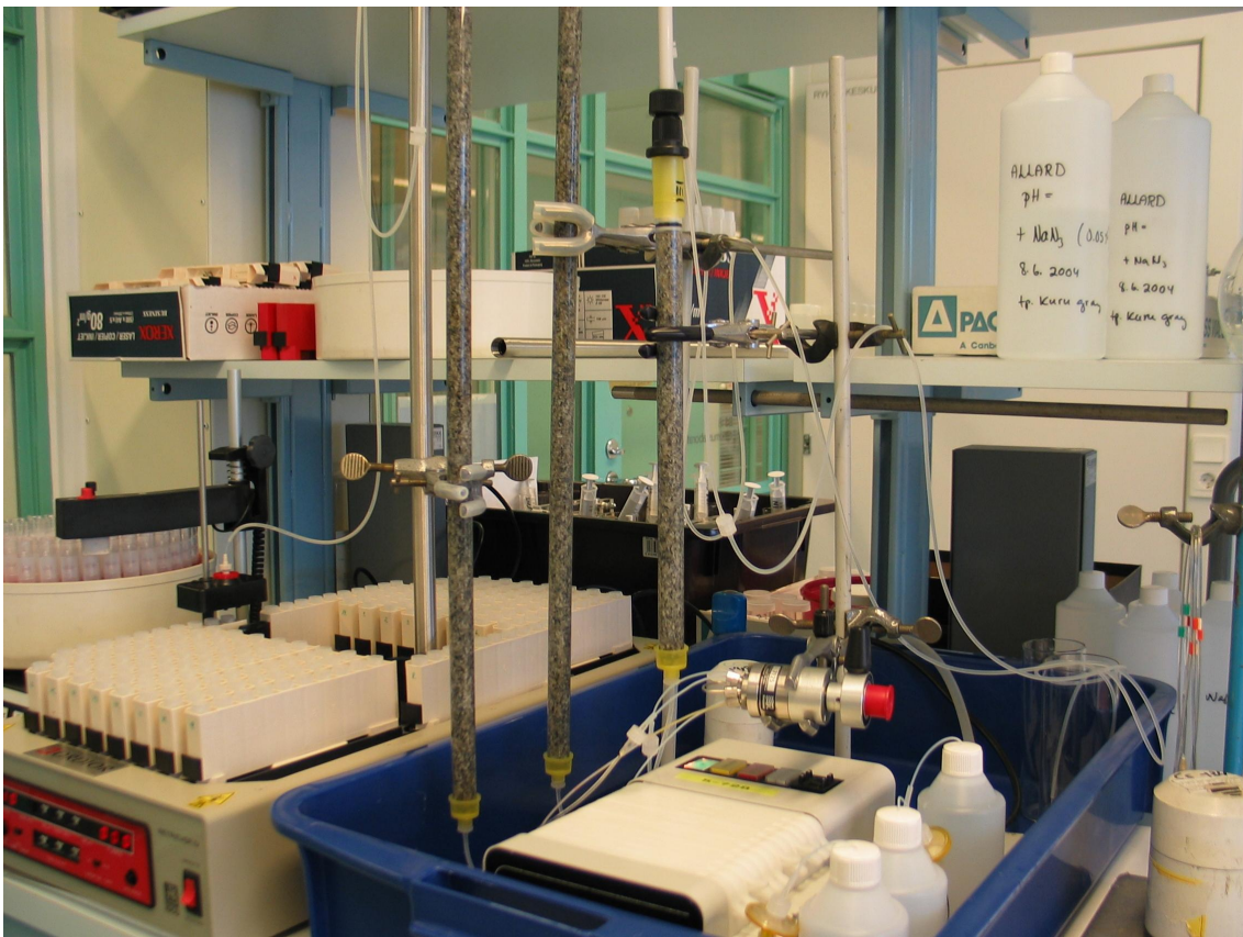
Figure 5-1. Borehole cores were used for rock columns. Tracer tests have been carried out using the columns.
