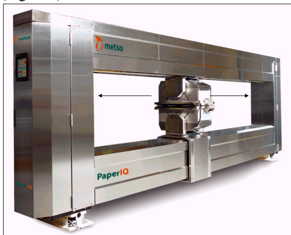
Figure 1. Measurement frame. The instruments are located in the moving scanner at the center of the frame. Paper moves through the frame between the upper and lower scanner heads. The arrows indicate the direction of the scanning (orthogonal with respect to the movement of the produced paper). (Courtesy of Metso).
