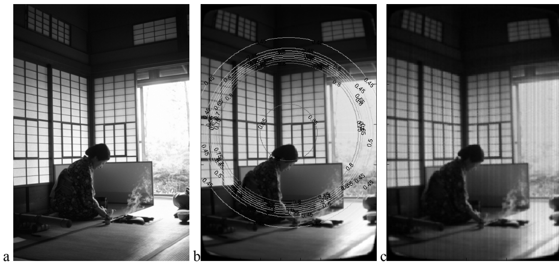
Figure 2. Simulation example. a - original image, b - image shown through a lens; values of the subjective quality factor are shown as contours on top of the image, c - image shown through a lens and detected with a CMOS detector.
