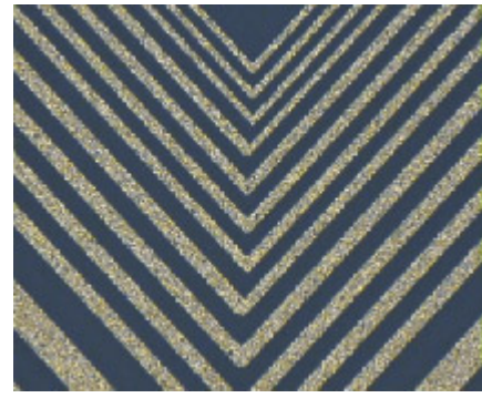
Figure 3. The optical microscope photo of etched conductors on DP951 tape. The narrowest lines are 40 \mu\text{m} wide.
