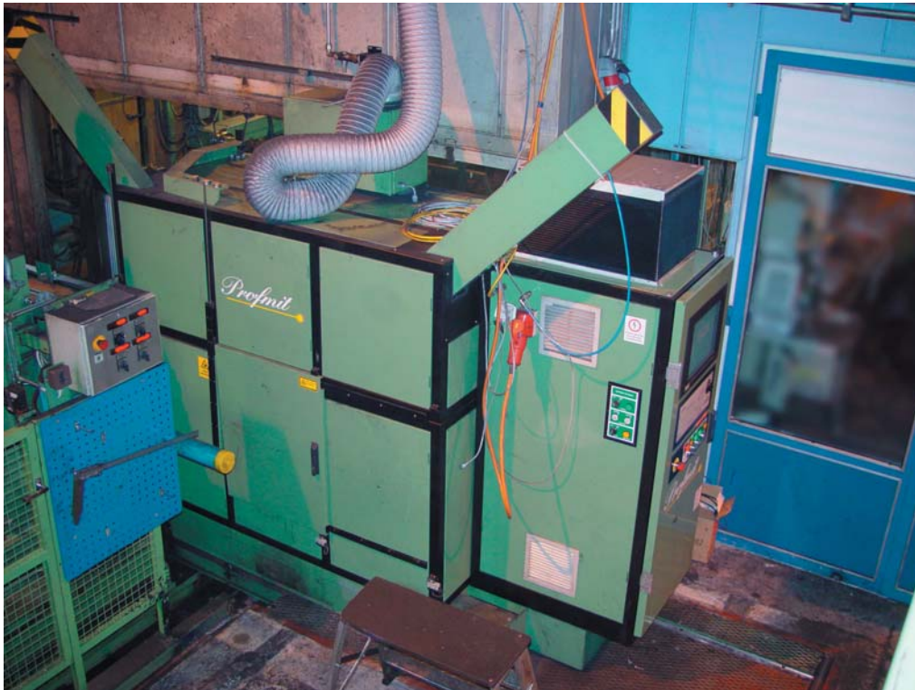
Figure 2. PROFMIT-measuring system has been installed into steel production line.
