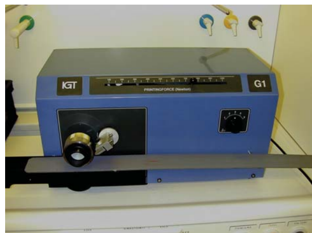
Figure 1. Tabletop gravure printability tester for material modification and first printing trials.
