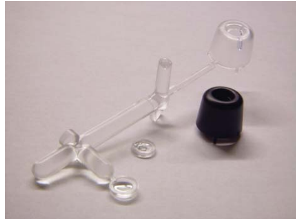
Figure 11. Injection moulded parts: clear lens, black holder and a test piece with both components.
