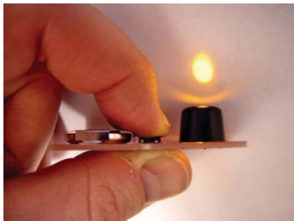
Figure 13. The module produces a round and nearly collimated illumination beam.
