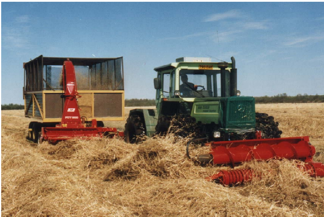
Harvesting of reed canary grass in spring (in May) by precision chopper on cut over peatland. (Photo: VTT Processes)
