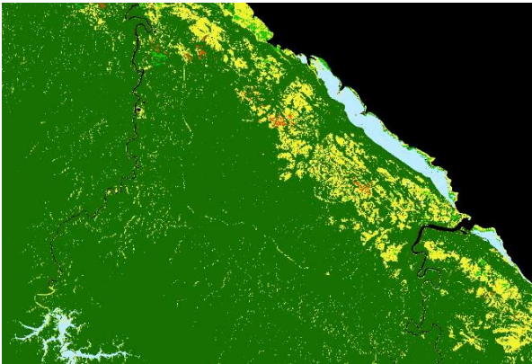
Figure 2. Autochange result of change classification 1993-2004. Input ERS data processed with the PGS (Envisat) processor. Red: from forest to non-forest, Dark green: forest in both years, Light green: from non-forest to forest, Yellow: non-forest in both years, Light blue: from forest (or mangrove) to water. Scattered yellow dots are due to the residual intensity variation, which is caused by inaccuracies of the DEM in the topographic normalization
