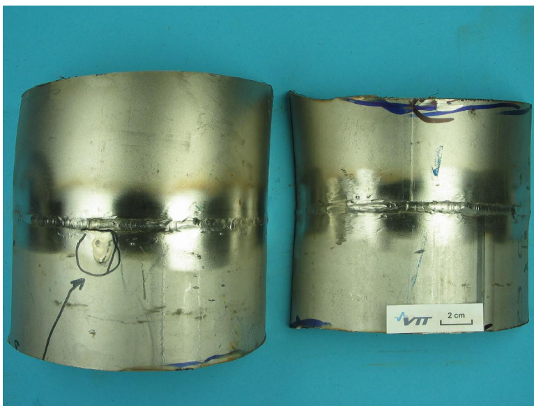
Figure 10. A perforated pit marked with an circle and an arrow on the outer surface of sample no 3.
