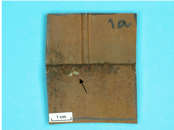
Figure 3. Starting pitting (an arrow) on the heat affected zone of a weld of sample 1.
