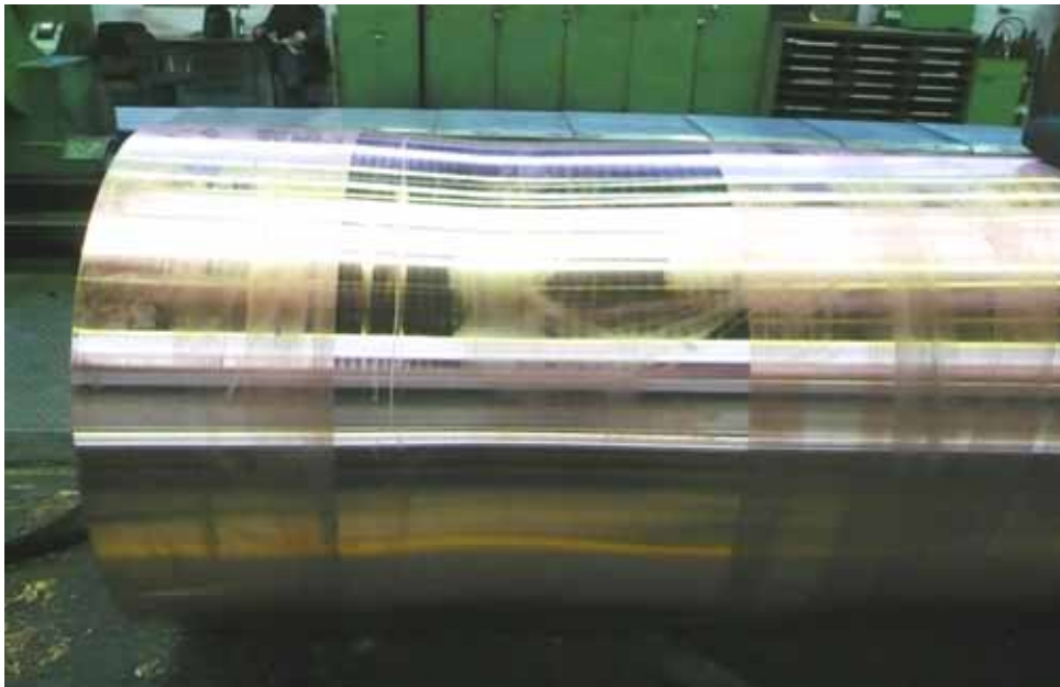
Figure 7. The material faults in the top part of the T55, above. The machined cylinder after repair removal of the faults, below.
