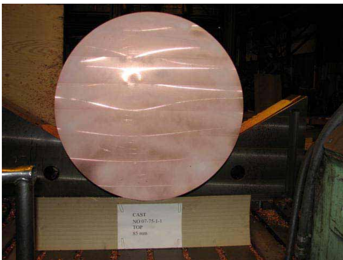
Top of ingot after the 85mm end machining, Photo No 1149
