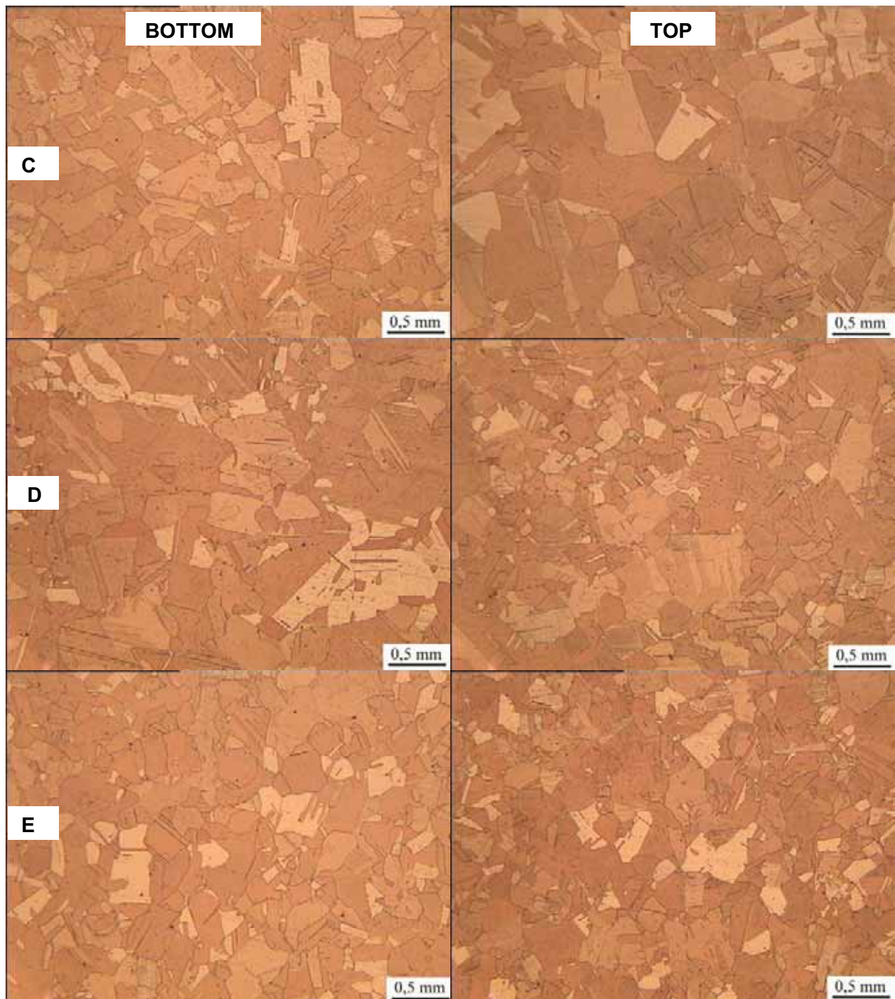
Figure 11. Microstructure from sample C (upper - bottom/top), D and E. 32x
