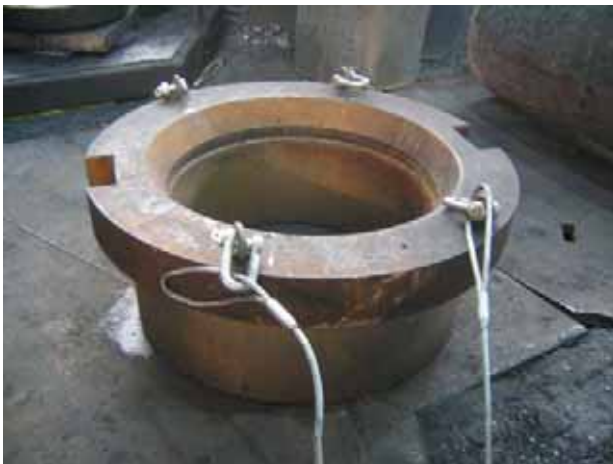
Figure 11. The centralization tool (tool id 855 mm, length of the straight part 400 mm).
