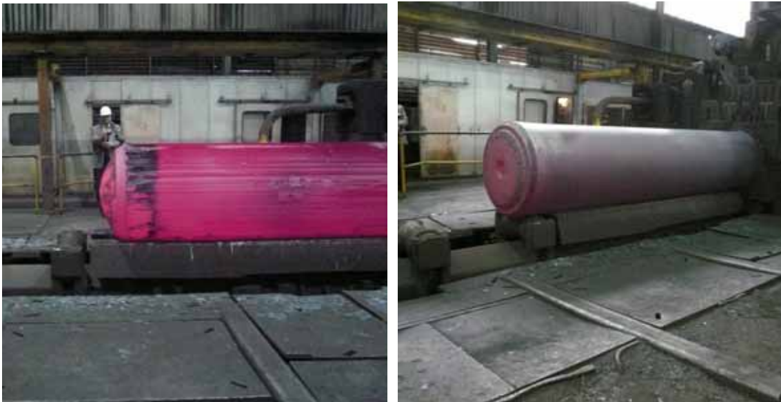
Figure 10. Bottom was deformed after the fifth draw. On the left, T55 bottom after pressing with the spherical mandrel, and on the right, after deformation with the new device shown in Fig. 9. (Vallourec & Mannesmann Tubes).
