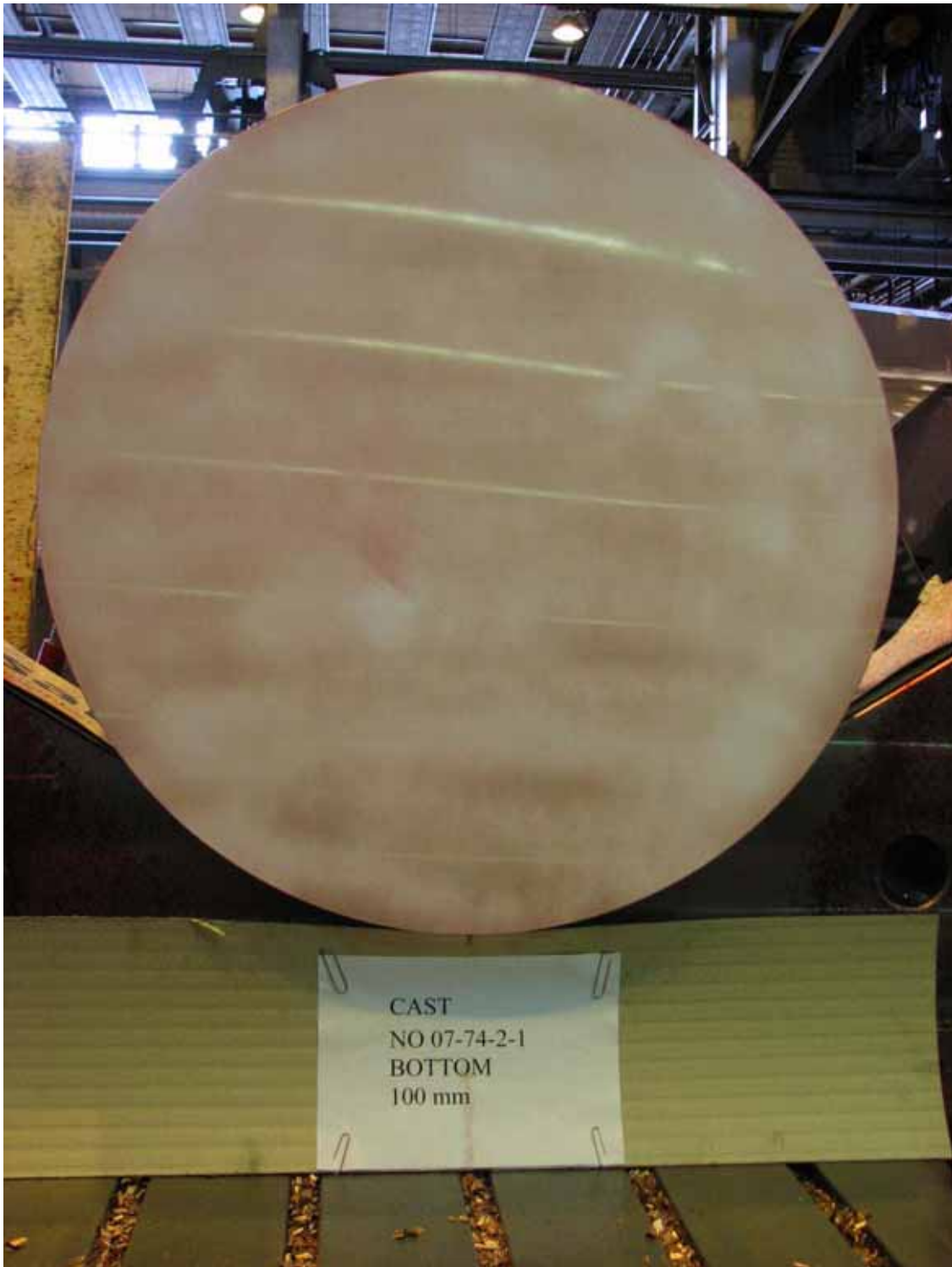
Bottom of ingot after the 100 mm end machining, Photo No 1144
