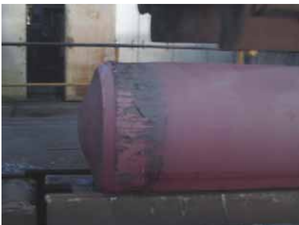
Figure 7. The tube bottom after first deformation of the bottom.
