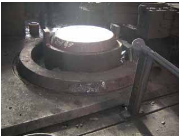
Figure 14. The work piece after swaging.
