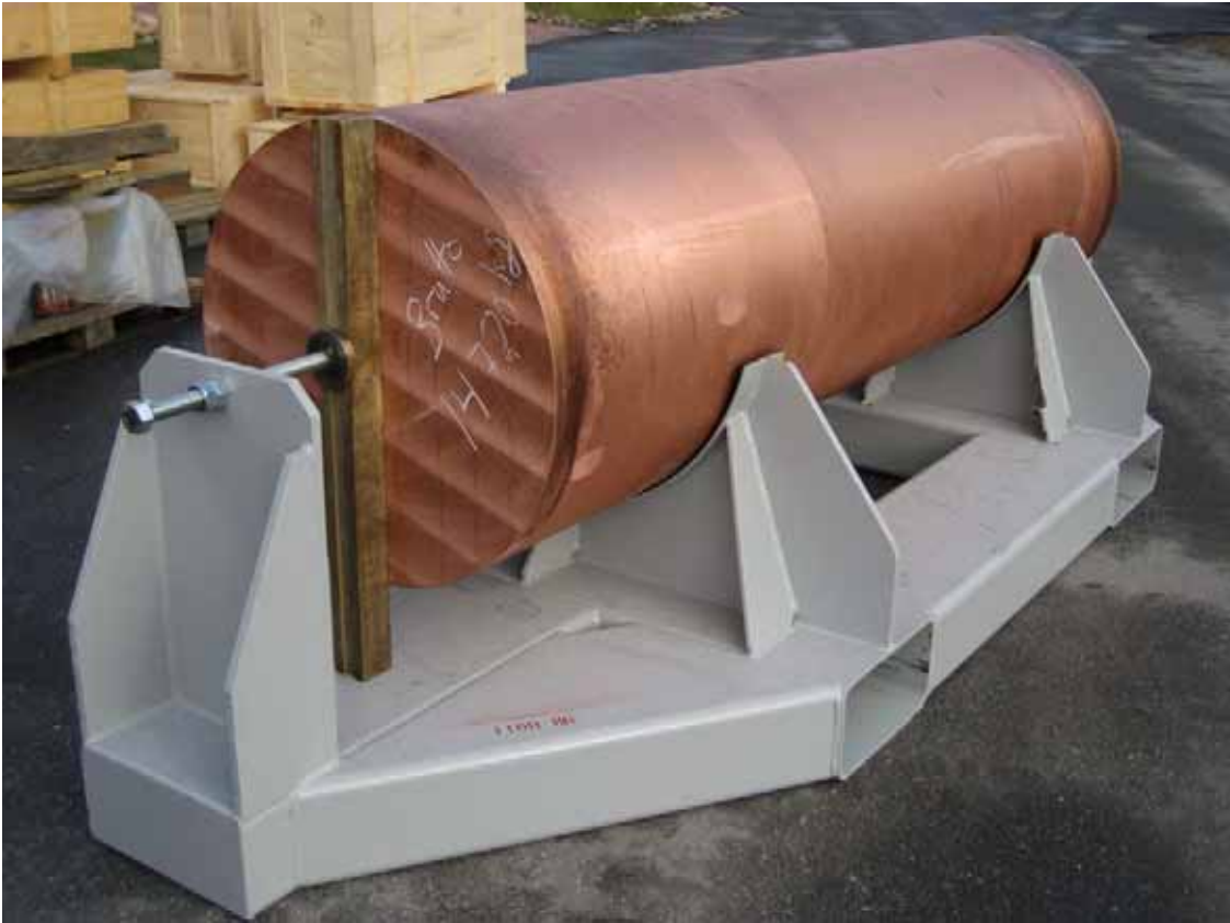
The ingot after the machining and grinding ready for delivery, Photo No 1717
