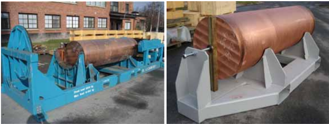
Figure 1. The billets for T54 and T55 ready for transportation to hot forming at Luvata Pori Oy.
