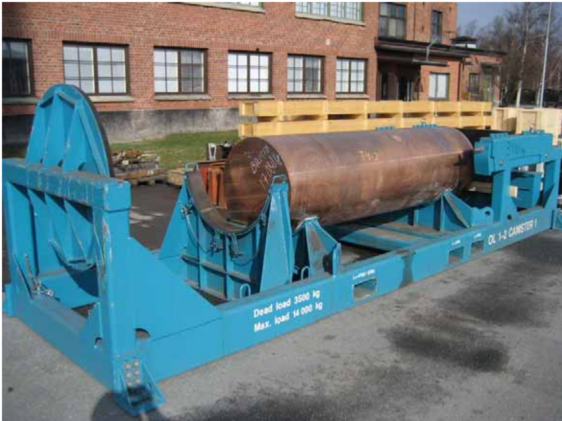
The ingot after the machining and grinding ready for delivery, Photo No 1719
