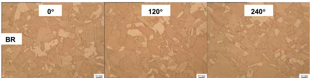
Figure16. T54 base ring microstructures at 0°, 120° and 240° circumferential position. 75x
