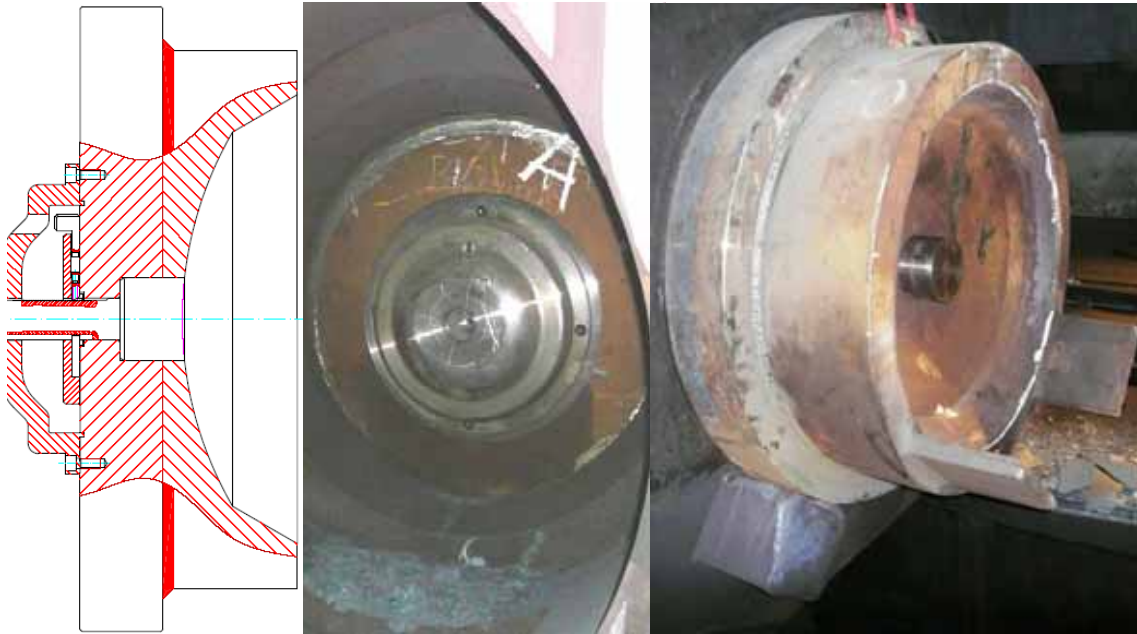
Figure 9. The new deformation device used for the bottom end deformation of the T55. (Vallourec & Mannesmann Tubes).
