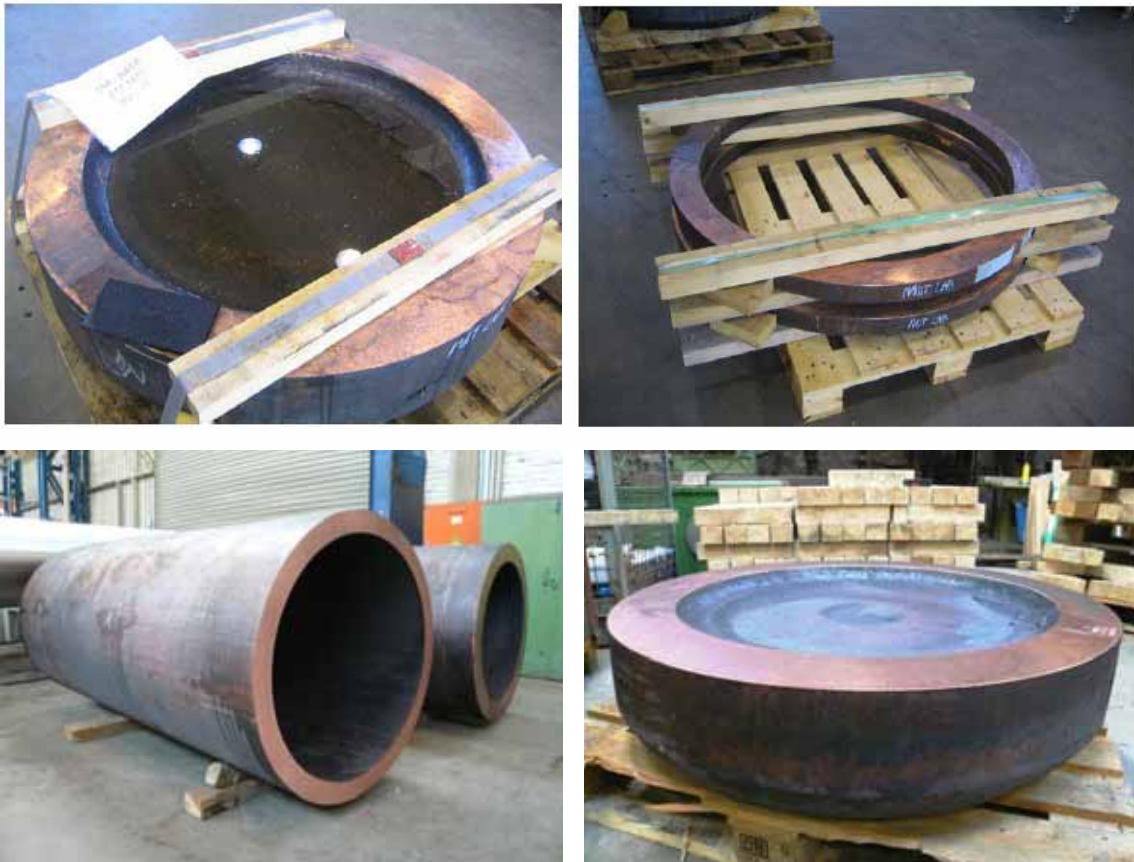
Figure 14. The copper shell pieces from the T54 (upper) T55 (lower) after cutting the sample rings.
