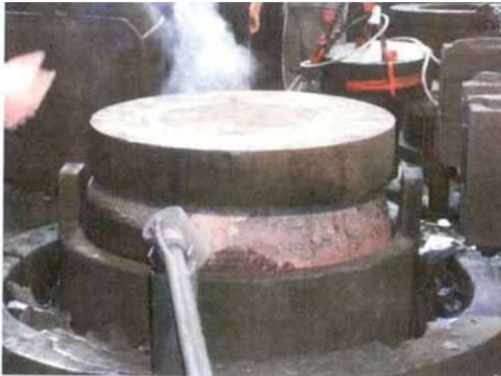
Figure 4. Uneven filling of the mould after swaging.
