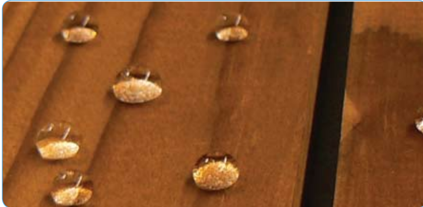
Figure 1. Nano-coating prevents water entry to wood and permits water vapor movements.
