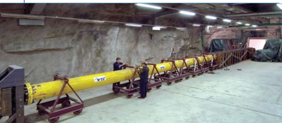
Figure 1. Impact test facility (pressure pipe, acceleration tube, piston catcher and force plate or impact wall).
