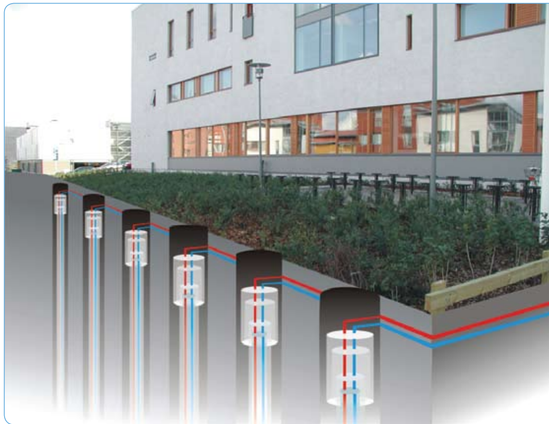
Figure 1. The bedrock cooling system of Ruusutorppa school in Espoo.
