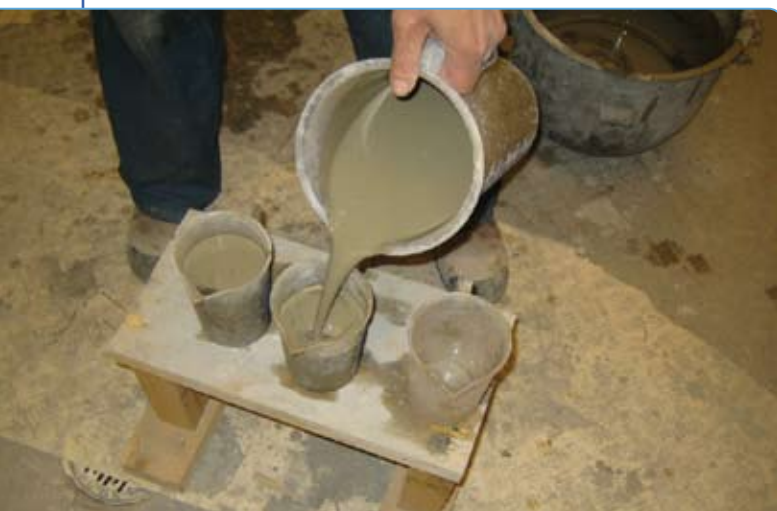
Figure 1. Freshly mixed rock injection grout ready for testing: flowability, injectability, setting time and strength properties.
