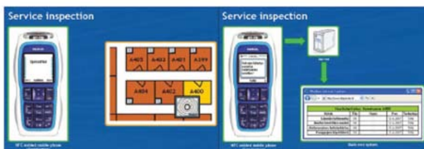
Figure 1. Principle of service and quality management of maintenance work using mobile application (e.g. cleaning and building maintenance)
