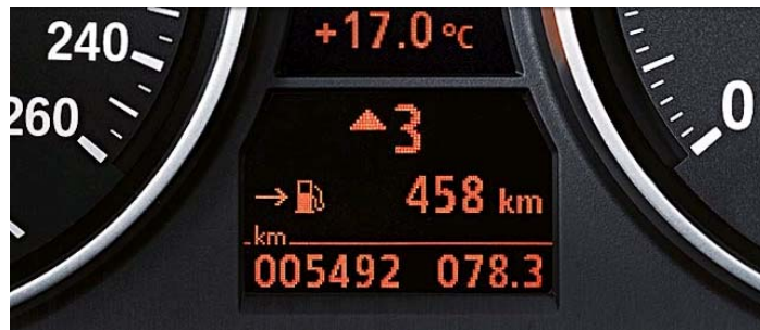
Figure 6: Example of a gear shift indicator on a vehicle instrument panel
