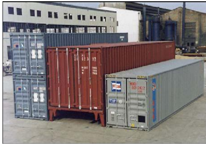
Figure 8. SECU box with standard containers.
