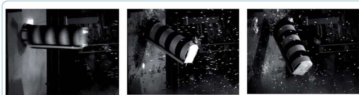
Figure 2. Still images of steel missile crash in impact test.
