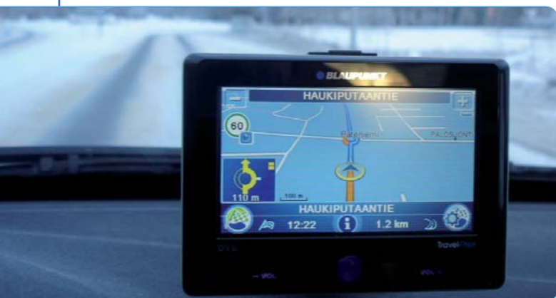
Figure 1. A personal navigation device as used in the TeleFOT benchmarking tests. With its camera this device detects the road-side speed limit signs and conveys the information to the display.
