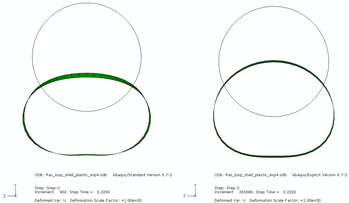
Figure 31. Cross-sections at time instants 0 and 0.22 s after the pipe break at the position slightly left from the restraint. The implicit analysis result (SPI) on the left, explicit on the right (SPE).
