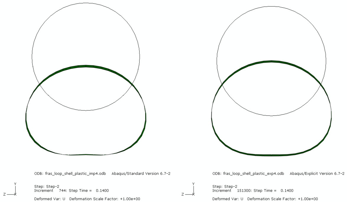
Figure 30. Cross-sections at time instants 0 and 0.14 s after the pipe break at the position slightly left from the restraint. The implicit analysis result (SPI) on the left, explicit on the right (SPE).
