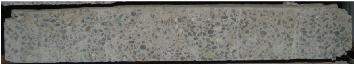
Figure 70. Quarter section of the test wall 644 cut at the centre line.
