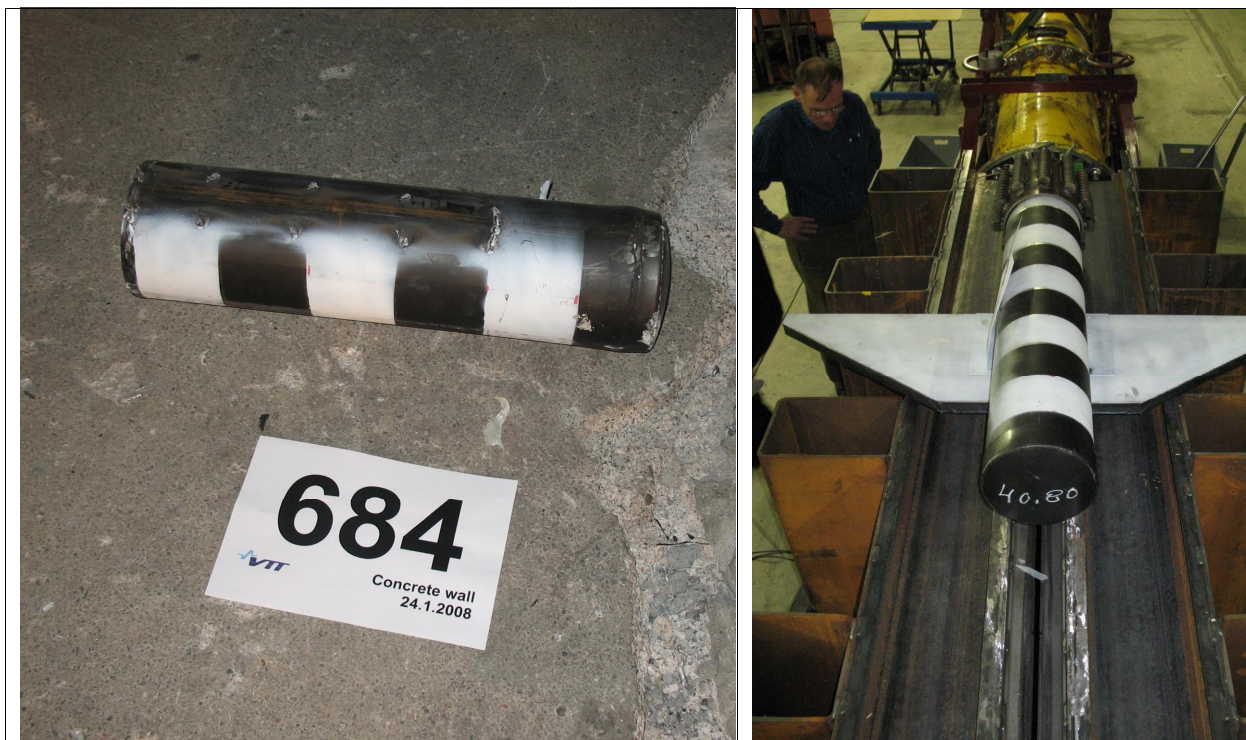
Figure 3. The rigid steel pipe missile with a diameter of 150 mm (left) and an aeroplane model with wings (right).
