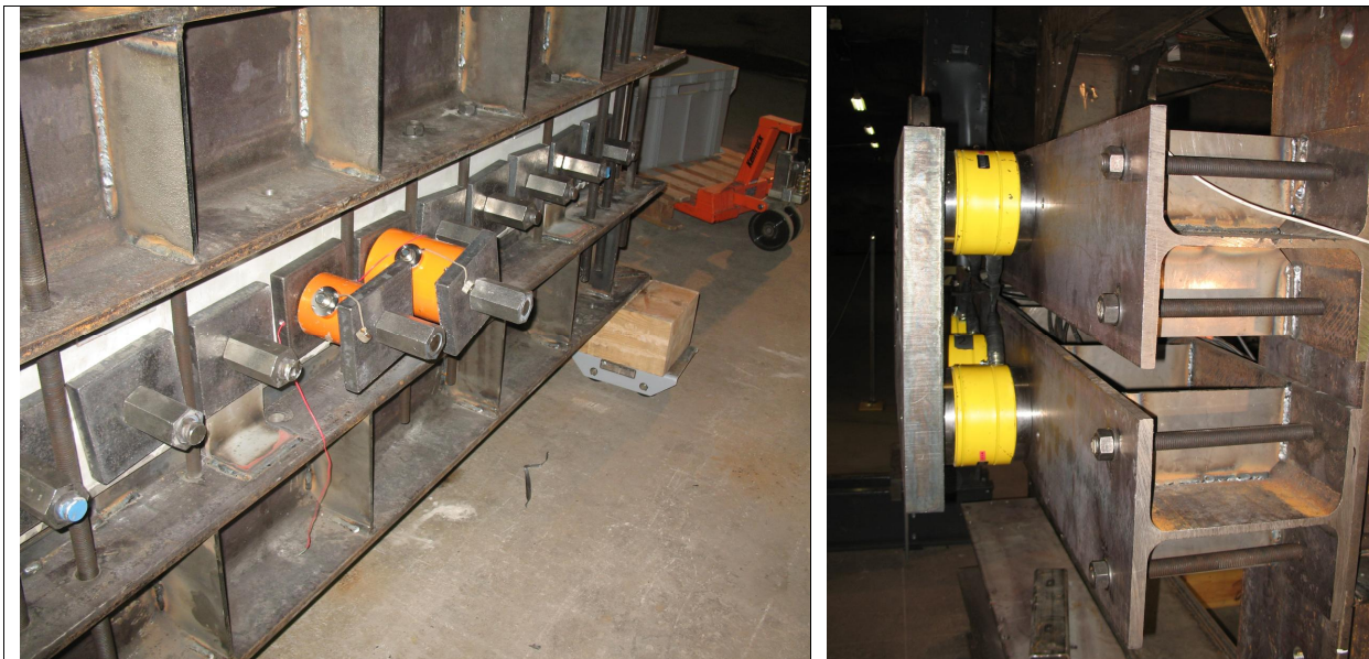
Figure 7. The force transducers of Dywidag bars (left) and the force transducers behind the force plate (right).
