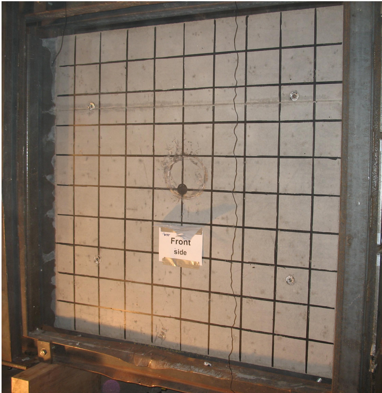
Figure 76. Front surface of the wall after test in Test 663.
