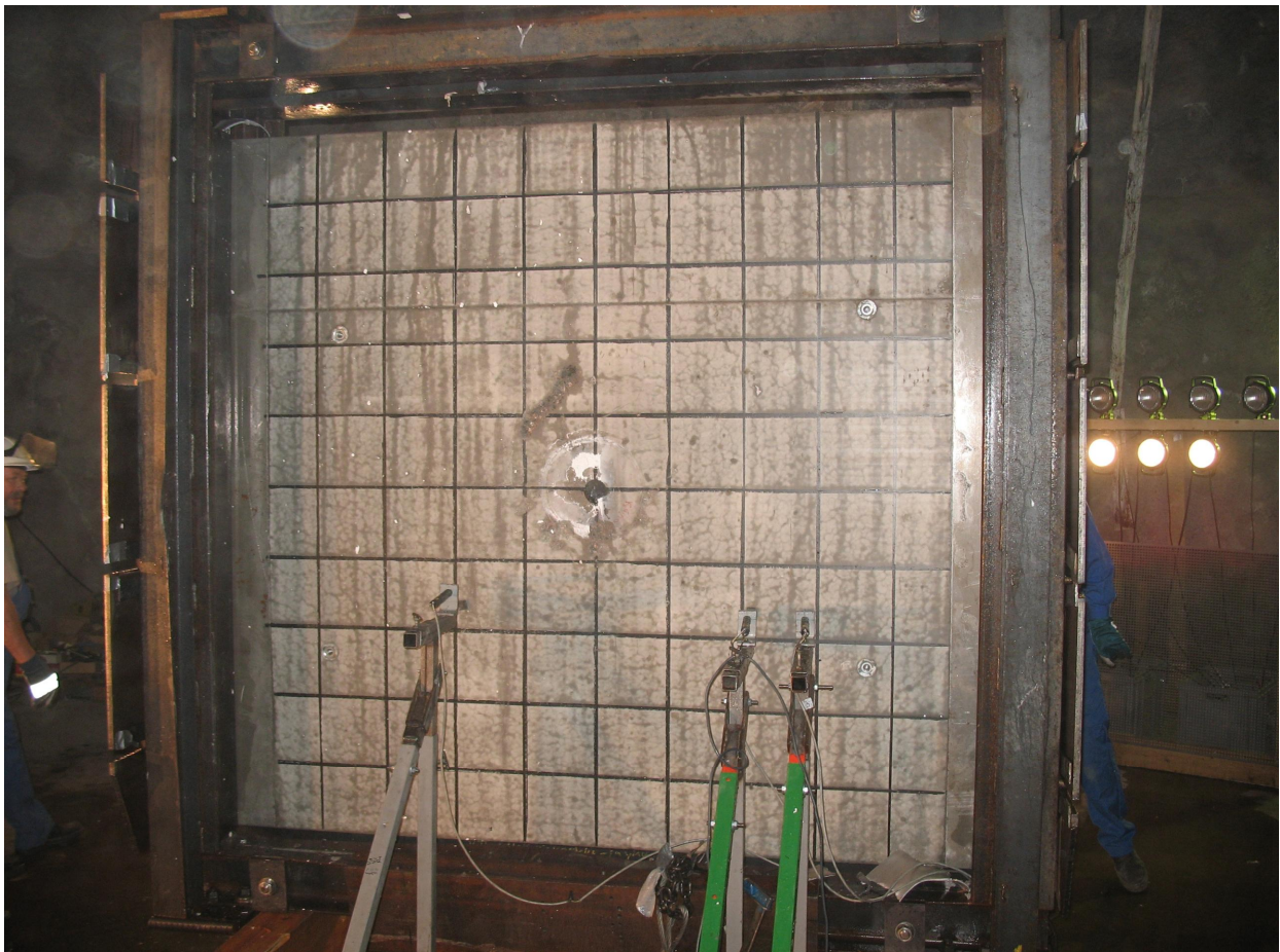
Figure 103. The front side of the wall after Test 650.
