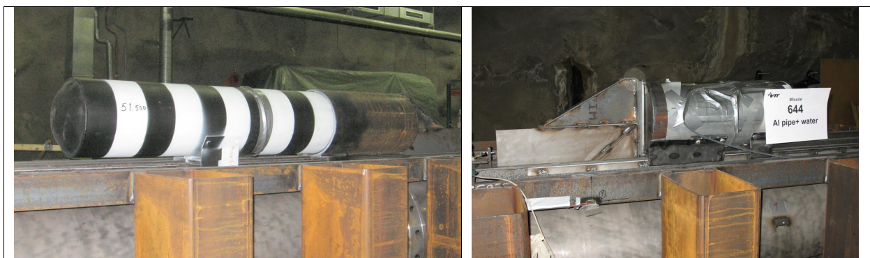
Figure 2. Dry (empty) aluminium (Al) pipe missile and wet (water filled) missile.
