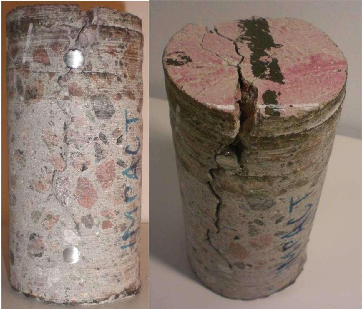
Figure 53. Sample specimen bored from the test wall 642.
