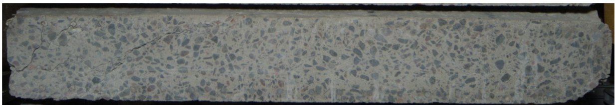
Figure 105. Quarter section of the test wall 650 cut at the centre line.
