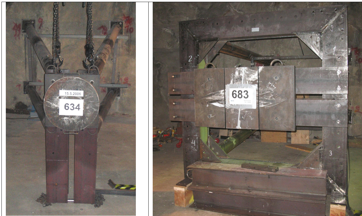
Figure 1. The second model (left) and third model of force plate construction.
