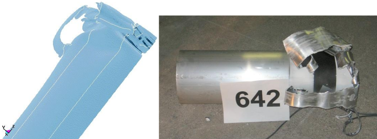
Figure 61. The deformed missile model and the actual deformed missile after the impact.
