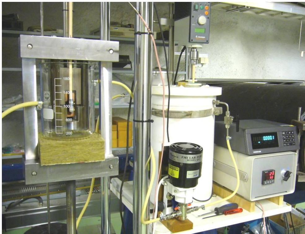
Fig 4. Multiaxial (CT) testing facility for combined creep and corrosion under simulated groundwater environment; specimen on the left (in the loading frame)
