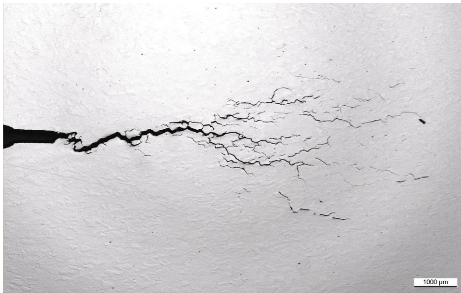
Fig 9. Crack branching in the second Cu-OF CT specimen after a test of 6200 hours.
