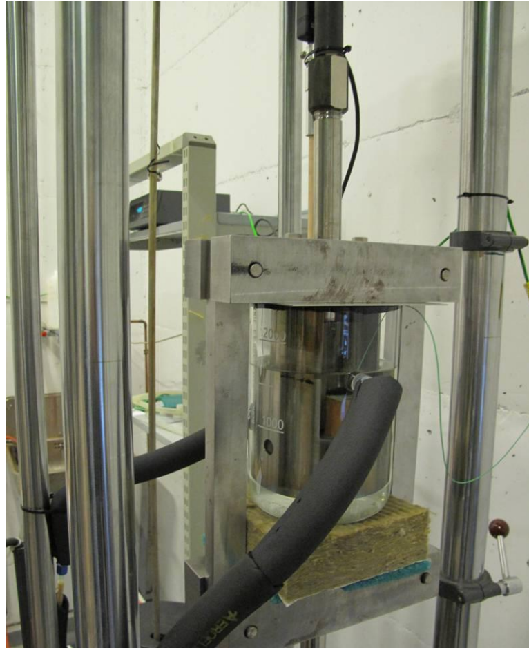
Fig 5. CT specimen in the test jar for the aerated groundwater environment in the new location.
