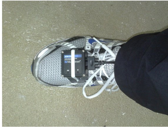
Figure 10. IMU (Microstrain 3DM-2GX) attached to a shoe.
