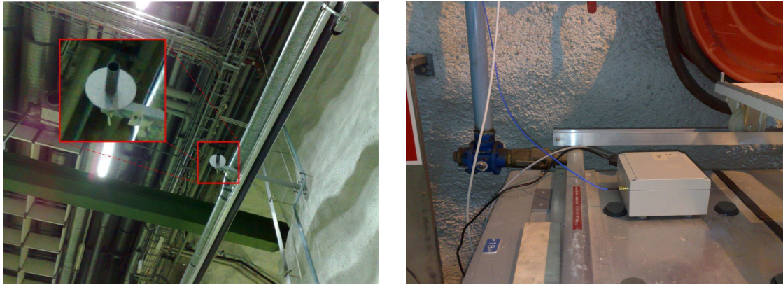
Figure 32. The large helix antenna (left) and the signal generator (right) of the pseudolite number 4.
