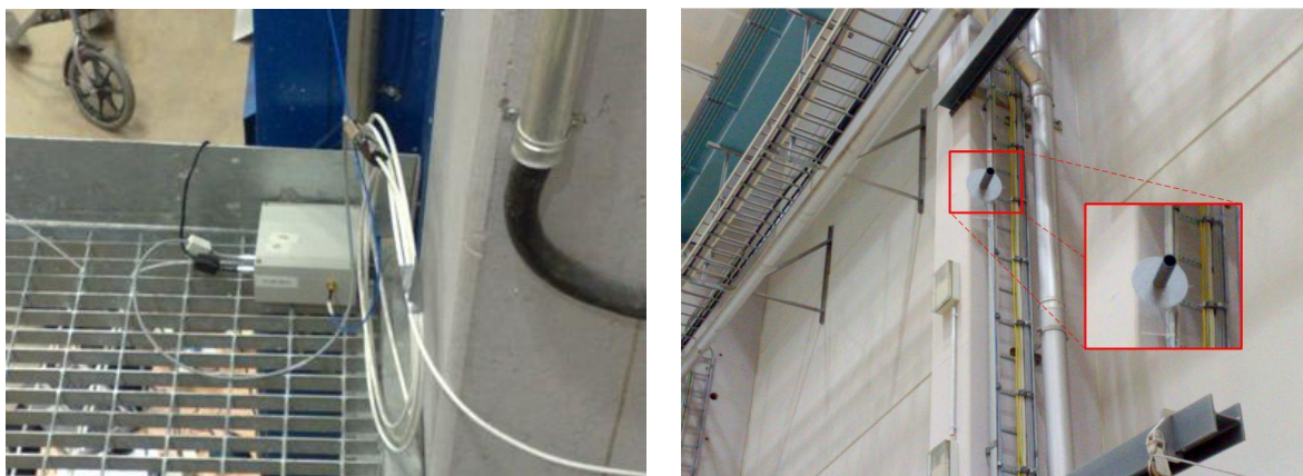
Figure 52. The signal generator of the pseudolite number 3 (left) and the large helix antenna of the pseudolite number 4 (right).
