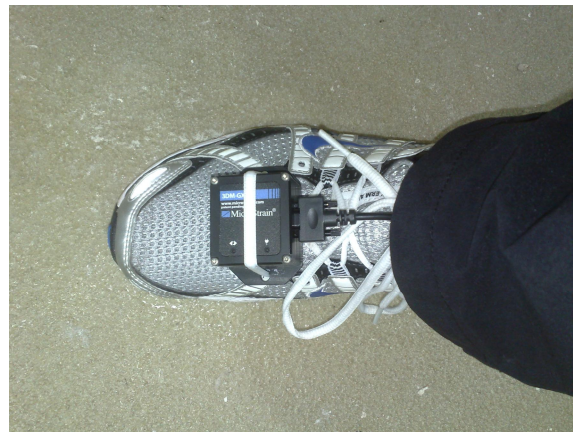
Figure 54. IMU (Microstrain 3DM-2GX) attached to a shoe.
