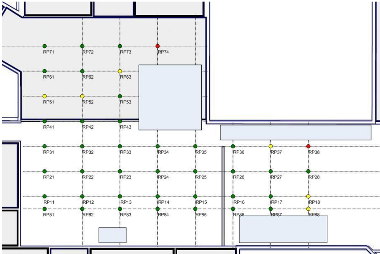
Figure 34. Reference points used to collect position estimates. Green colour shows the best operating range of the pseudolite position system using continuous signals, yellow a bit problematic areas and red the areas where reliable position estimates couldn't be reached.
