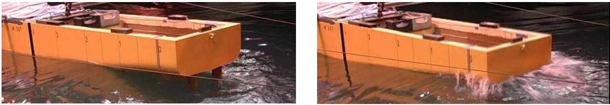
Figure 3.16. Stern of the Seatech-D model in hogging (left) and sagging (right) conditions in regular head waves at zero speed, \omega = 0.60 rad/s and wave amplitude a = 3.0 m in full scale.
