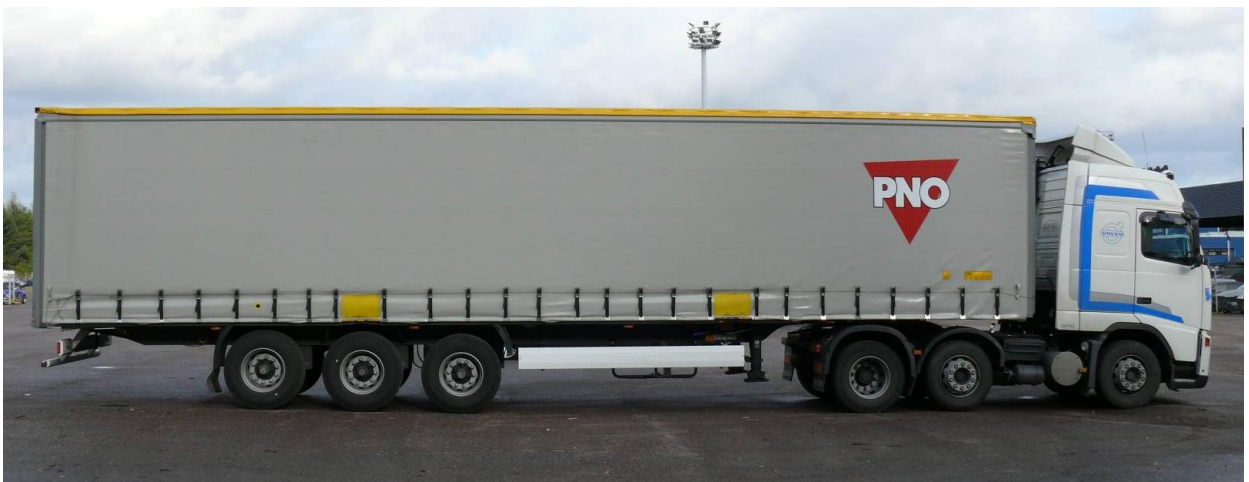
Figure 4.2 A 42 ton combination, Volvo FH 440 and a semi trailer
