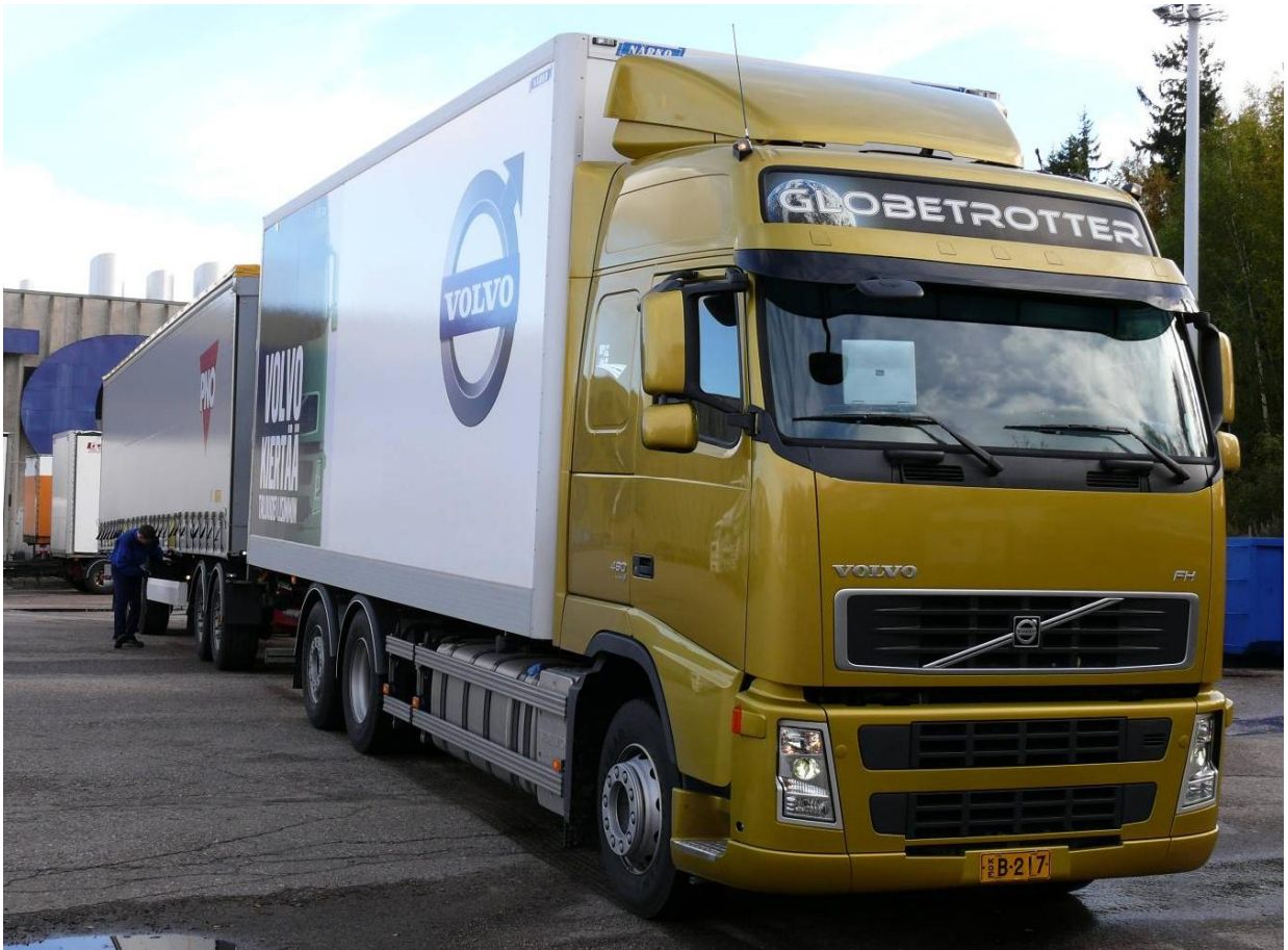
Figure 4.3. A 60 ton combination, Volvo FH 480 and a semi trailer connected by means of a dolly
