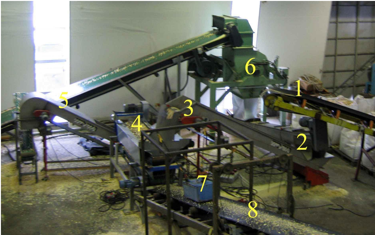
Figure 9. Continuous cleaving and screening process for pulp chips. 1 = feeding of pulp chips, 2 = conveyor of cleaved chips, 3 = feeding pulp chips and cleaved chips on screen, 4 = Pocket Roll screen, 5 = conveyor of oversized chips, 6 = knife-mill, 7 = magnet, 8 = conveyor of accepted pin chips.
