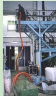
Figure 4. Pneumatic conveyor is flexible and it could lift pellets to the height of 3.5 meters easily. Length of the tube was 12.5 m.
