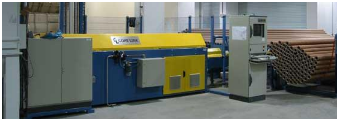
Figure 2. Automated core cutter 3 .
