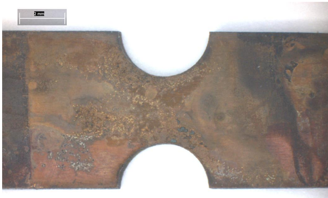
Figure 6: Stereomicroscopy image of bar Cu6, which had been tested at a constant load of 250 MPa.
