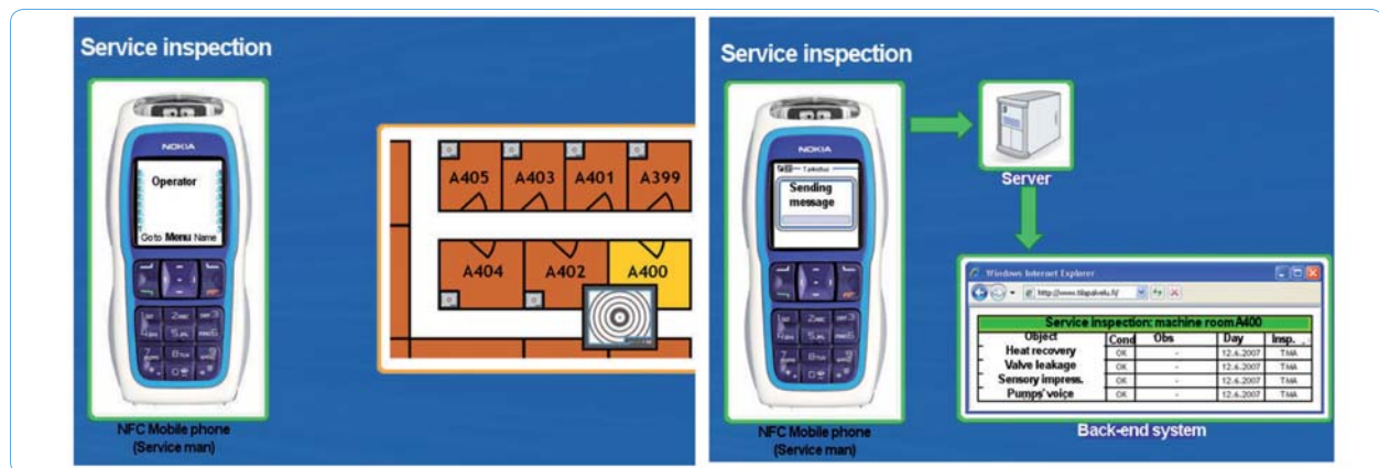
Figure 1. Principle of service and quality management of maintenance work using mobile application (e.g. cleaning and building maintenance).
