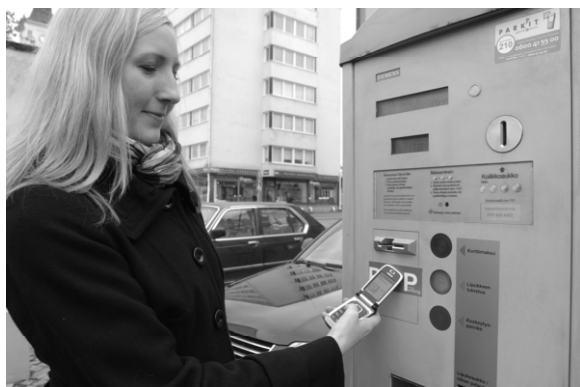
Fig. 5. A Parking zone selection by touching a zone tag (Picture copyright: Juha Sarkkinen).
