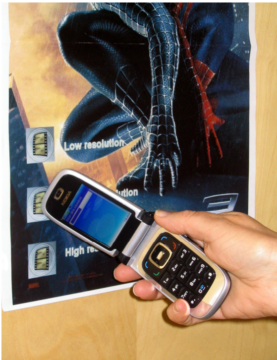
Fig. 9. The user is downloading a movie trailer from a memory tag attached to a poster. The mobile phone screen shows a progress bar displaying how much of the video clip has already been downloaded.
