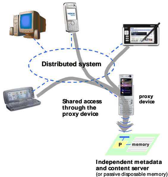
Fig. 6. Shared storage in a multi-device system. The mobile phone acts as a proxy device, connecting the passive memory tag with the network.
