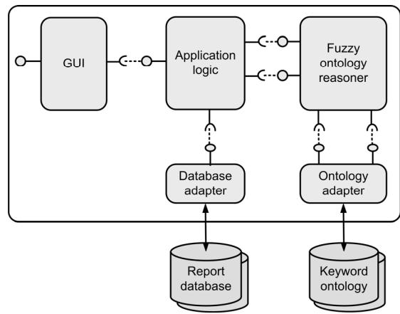
**Figure 3. Demo software components.**
