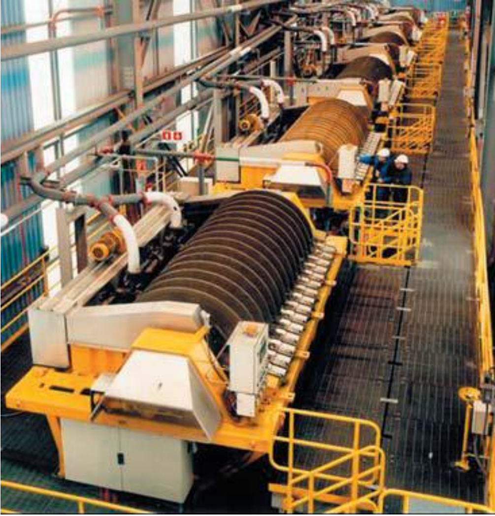
Figure 9. Industrial installation of Ceramec capillary filters which have ultrasonic cleaning system [10].
