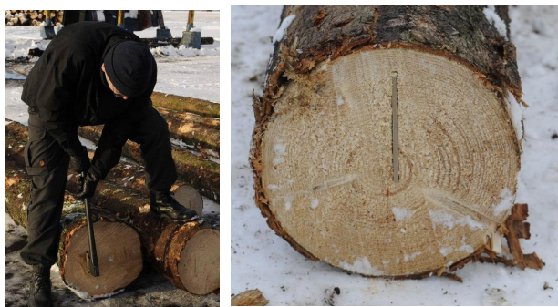
Figure 7. Manual transponder application and the applied transponder in the log end.
