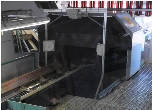
Figure 10. Reader antenna set-up at the log sorting.
