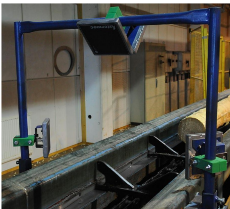
Figure 11. Reader antenna set-up at sawing.
