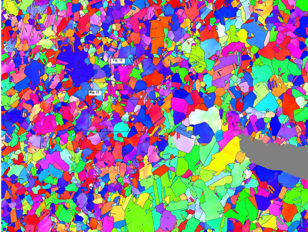
Fig. 10. EBSD grain orientation map IPF-Z, with locations of Figs 12-13 shown. The total width of the image is 1.07 mm; crack tip region shown in light grey.
