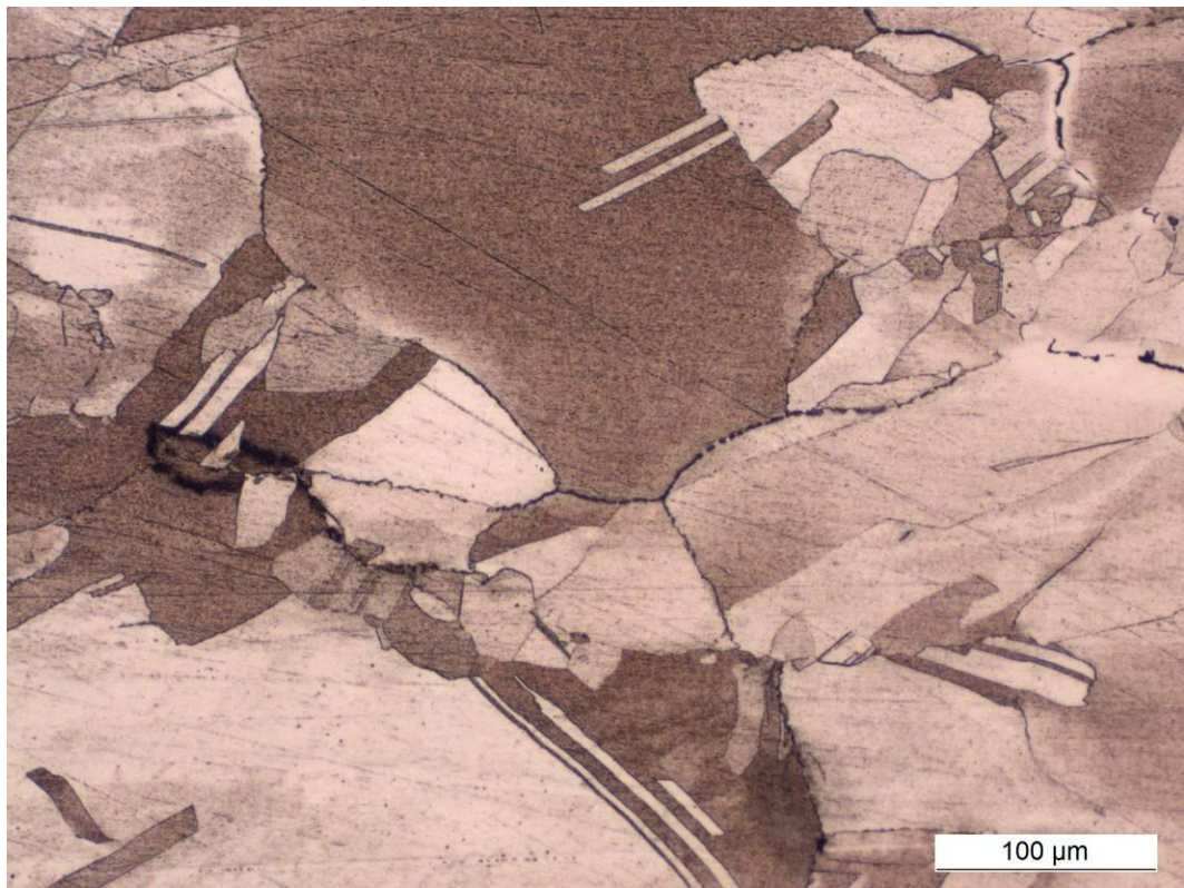
Fig 15. Grain boundary cracking in the third Cu-OF CT specimen after 8334 h of testing.
