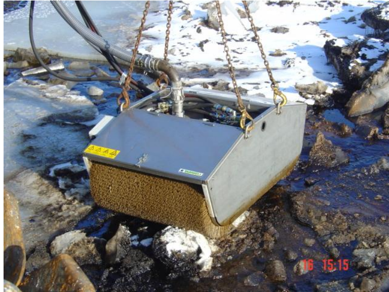
Figure 22. Lamor MABS in operation (Högström, personal communication, 20.1.2010).
