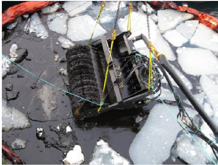
Figure 24. Testing of the LRB 150 skimmer during the experimental field trial in May 2008 (Singsaas, et al., 2008).
