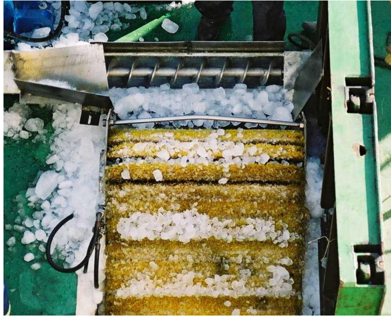
Figure 20. The brush-recovery system of the LOIS Ice Vibrating Unit (VTT, 2003).
