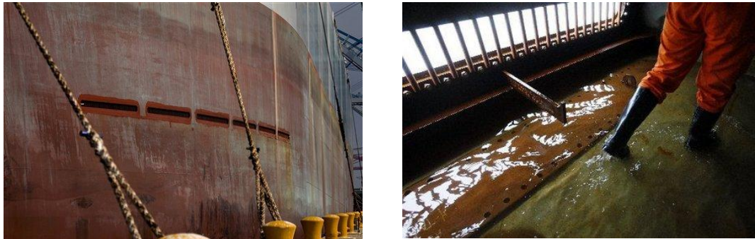
Figure 30. The intake vents on the side of the A Whale vessel (Associated Press, 2010).
