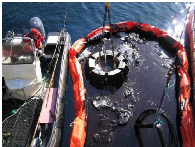
Figure 23. Testing of the Helix 1000 skimmer during the experimental field trial in May 2008 (Singsaas et al. , 2008)
