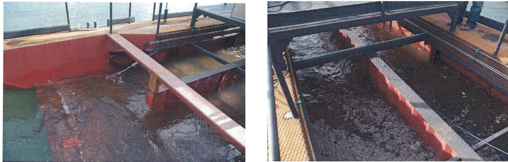
Figure 27. The intake (left) and recovery area (right) of the OilWhale vessel (Kappelinranta, 2010).
