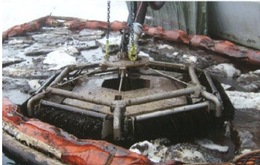
Figure 25. The Polar Bear skimmer in operation during the 2009 trials (Desmi, 2009).
