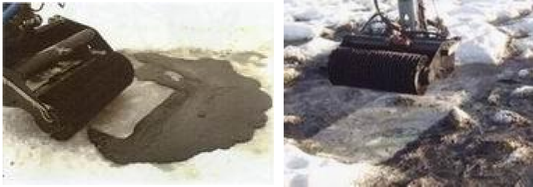
Figure 21. Oil recovery bucket in operation (SYKE, 2010a).
