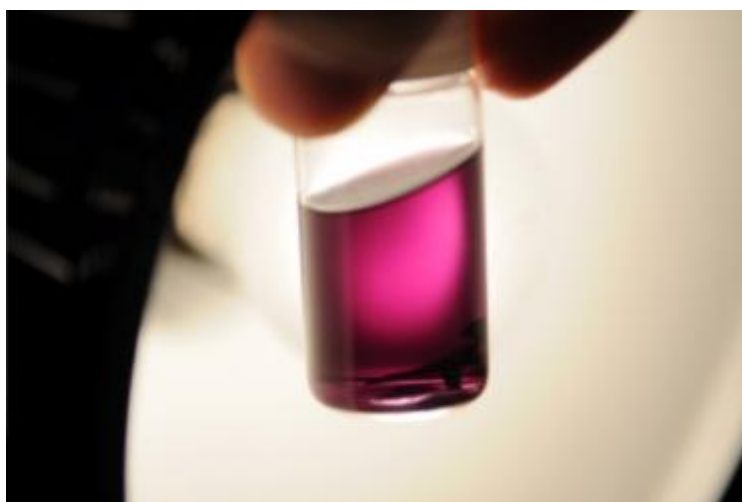
Figure 77. Gold nanoparticles in isopropanol solution.
