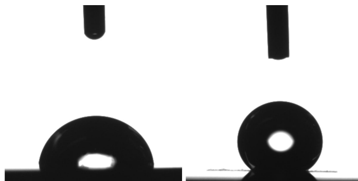
Figure 81. Contact angle measurement of the stainless steel surface. Value of 80^\circ is obtained for smooth surface and 152^\circ for structured surface.
