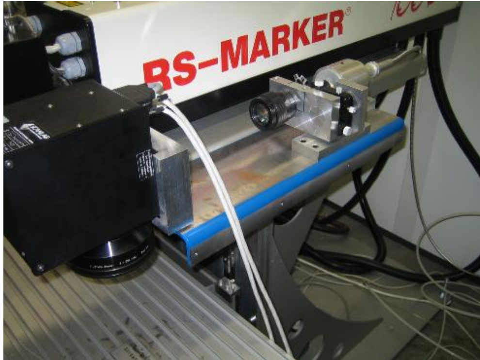
Figure 22. SPI fiber laser optical setup.
