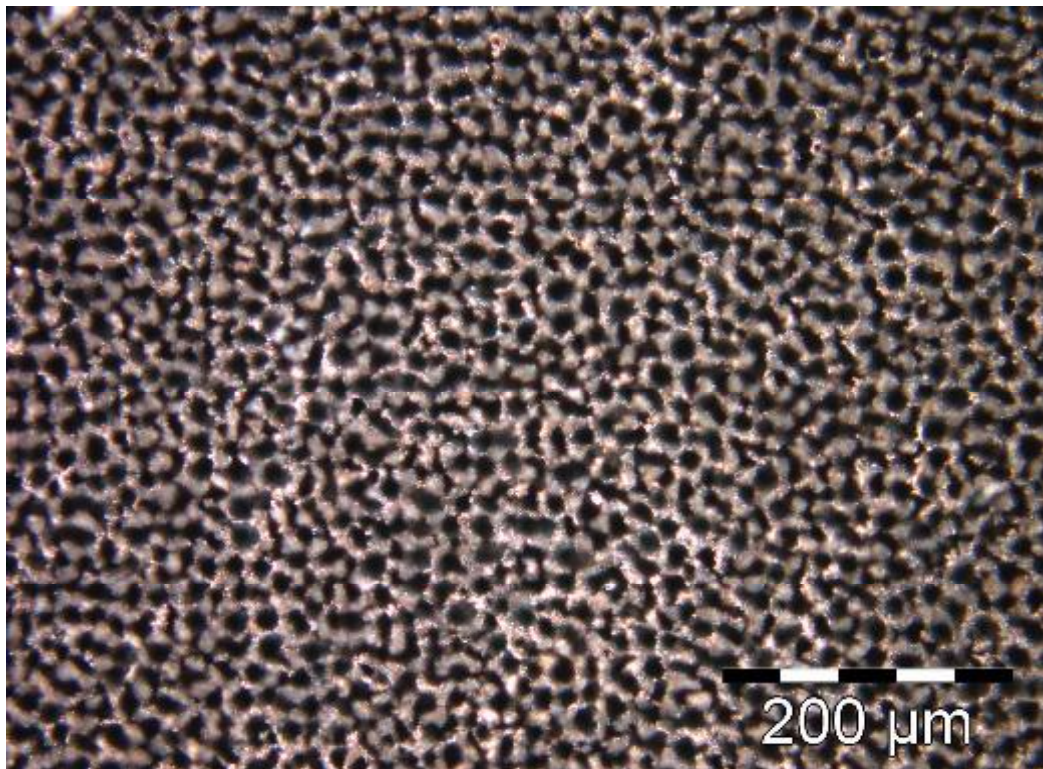
Figure 35. Power setting APT25, speed 1 mm/s, hatch distance 0.01
