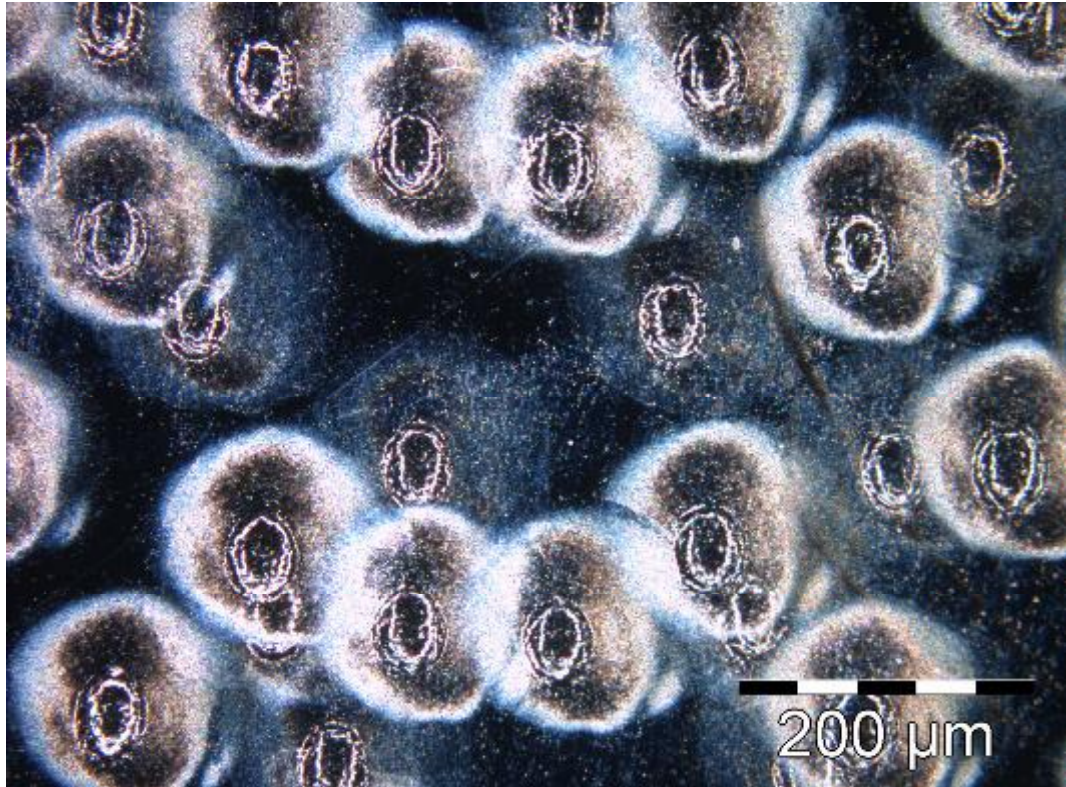
Figure 34. Power setting APT60 (full power), speed 320 mm/s, hatch distance 0.1 mm
