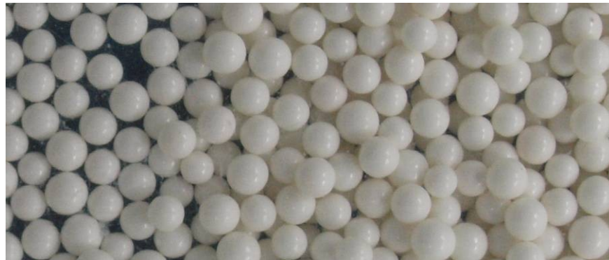
Fig. 6. The particle material is composed of ceramic beads ( \varnothing 0.8\text{-}1.0 \text{ mm} ).
