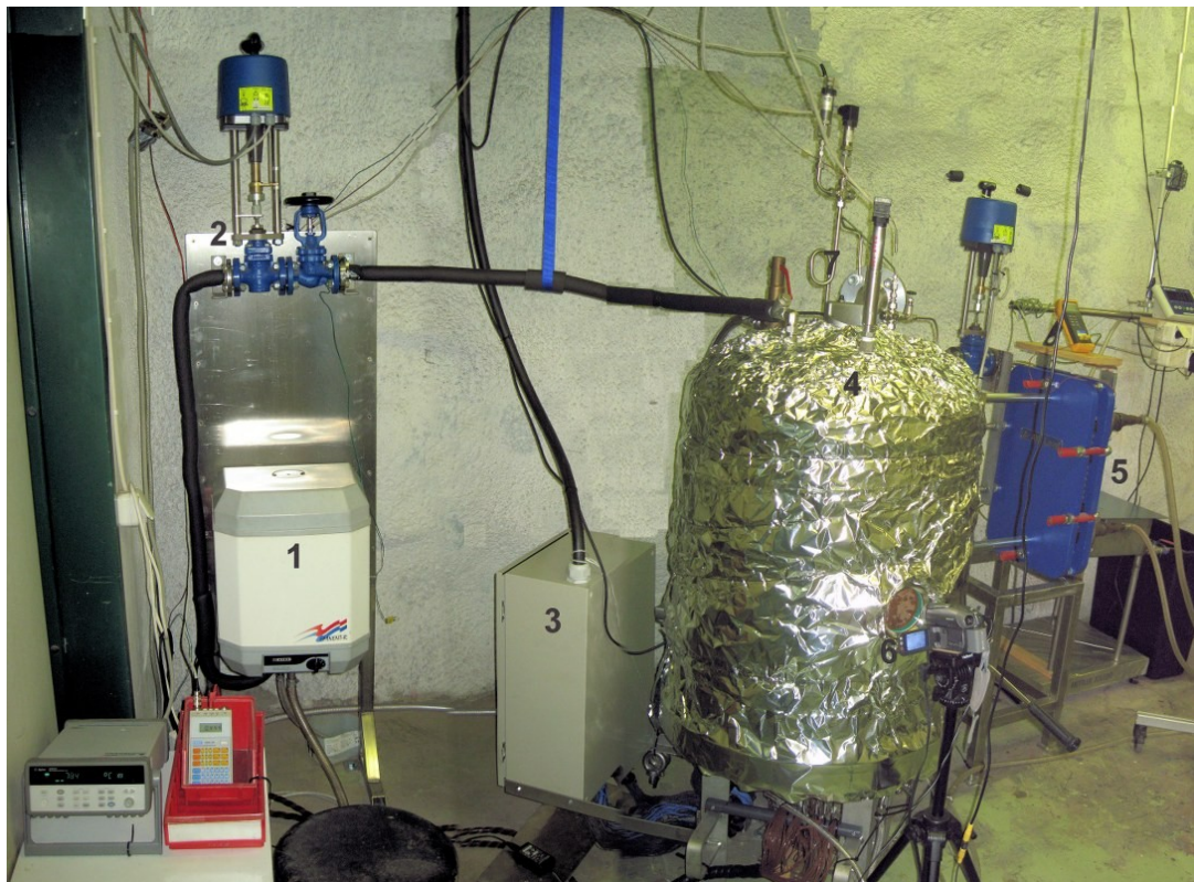
Fig. 1. COOLOCE test facility details, 1) feed water pre-heater (3kW), 2) feed water control valve, 3) input power connection box, 4) pressure vessel, 5) condenser, 6) video monitoring and recording, 7) water level control and pressure gauges.
