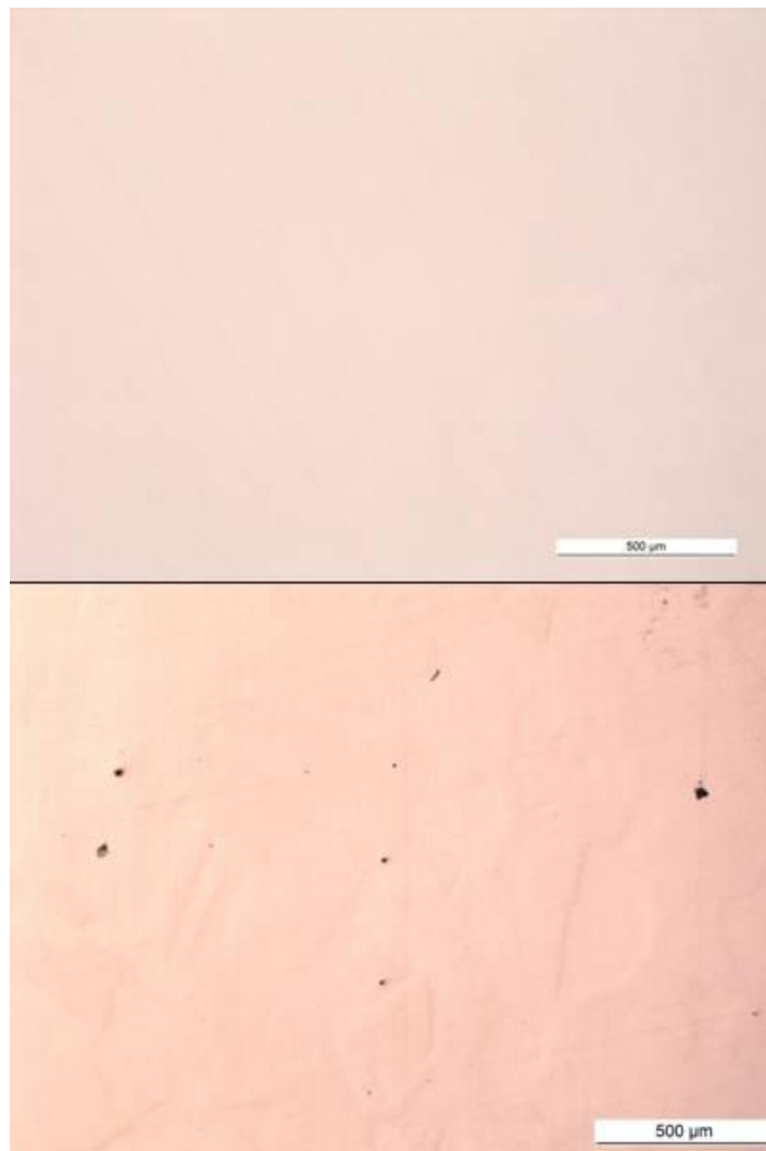
Figure 22. Comparison of polished surface of unexposed CuOFP and that of cross section 27.11 of slice Z1 in Fig. 21. Area fraction of inclusions is 6.5 \cdot 10^{-4} .
