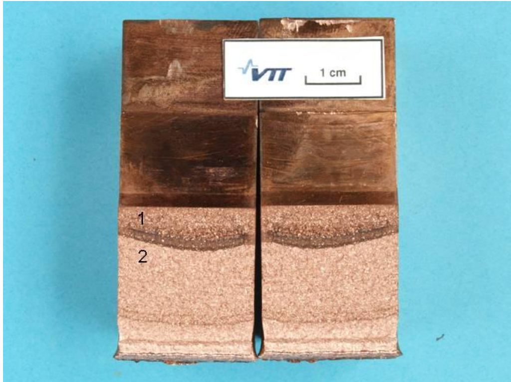
Figure 12a. A digital picture of the fracture surface, Test run 6 (N 2 /air). The prefatigue area (1) and afterfatigue area (2).
