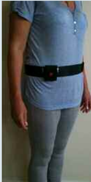
Figure 1: Subject wearing a wireless ambulatory monitor attached to a belt placed around the waist. The triaxial accelerometer in this device is used to characterize the subject's performance of a number of physical assessments and hence determine their risk of falling in the near future.
