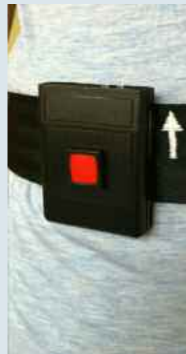
Figure 1: Subject wearing a wireless ambulatory monitor attached to a belt placed around the waist. The triaxial accelerometer in this device is used to characterize the subject's performance of a number of physical assessments and hence determine their risk of falling in the near future.
