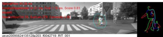
Fig. 9 Creation of pedestrian shape model bank,
