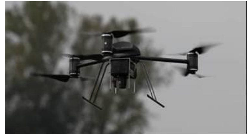
VTT proof-of-concept prototype used for test targets onboard Draganfly X6 UAS helicopter
