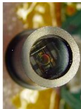
Detector modules including a Fabry- Perot interferometer detector and optionally cooling.
