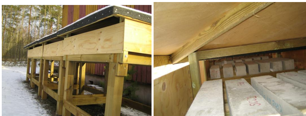
Figure 3. DuraInt field exposure site in an environment without salt in southern Finland (Otaniemi field, Espoo). Carbonation testing sheltered.
