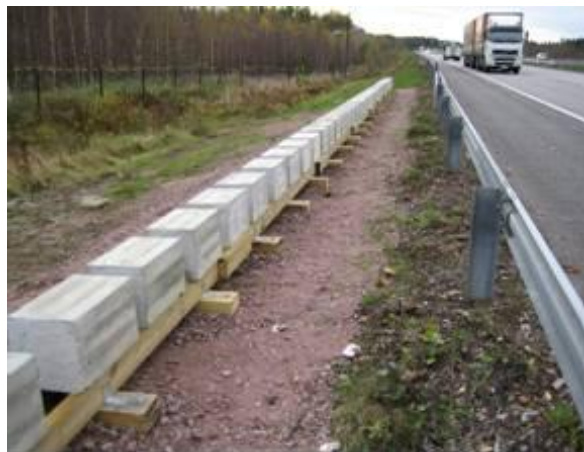
Figure 14. Specimen for chloride penetration studies at HW 7 field in Southern Finland (Kotka). A) At a distance of 4.5 m from the road lane. B) At a distance of 6 m, 8 m and 10 m from the road lane.
