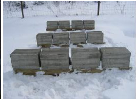
Figure 14. Specimen for chloride penetration studies at HW 7 field in Southern Finland (Kotka). A) At a distance of 4.5 m from the road lane. B) At a distance of 6 m, 8 m and 10 m from the road lane.
