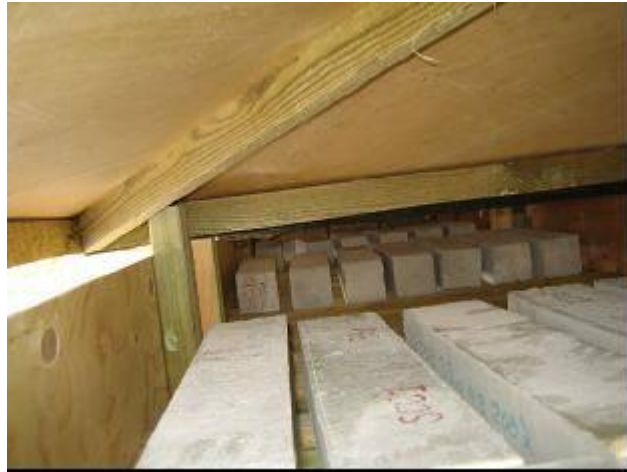
Figure 39. Specimen (beams 100x100x500 mm 3 ) in field sheltered carbonation exposure.
