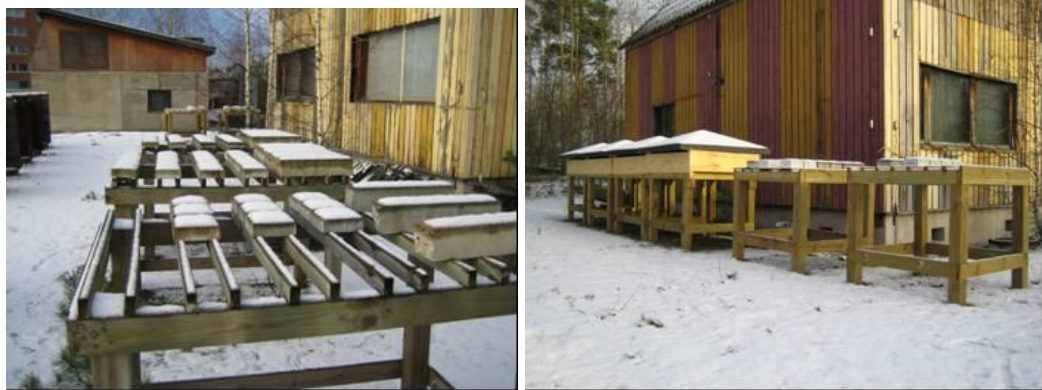
Figure 2. DuraInt field exposure site in an environment without salt in southern Finland (Otaniemi, Espoo).
