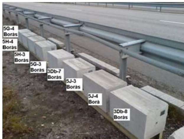
Figure 15. DuraInt specimen in Swedish testing field in Borås (2009).
