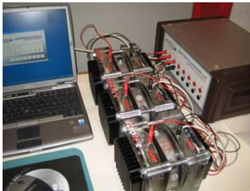
Figure 17. Measurement of chloride migration coefficient ( D_{nssm} ) [NT Build 492].
