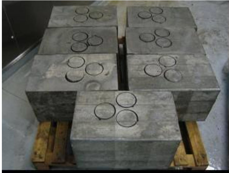
Figure 22. Surface treated specimens and reference specimen right after coring of three smaller specimens ( \varnothing 98 mm) per each specimen for laboratory measurement of migration coefficient ( D_{nssm} ).
