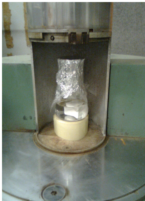
Figure 2. The position of painted concrete block sample in Gammacell 220 ready for irradiation.
