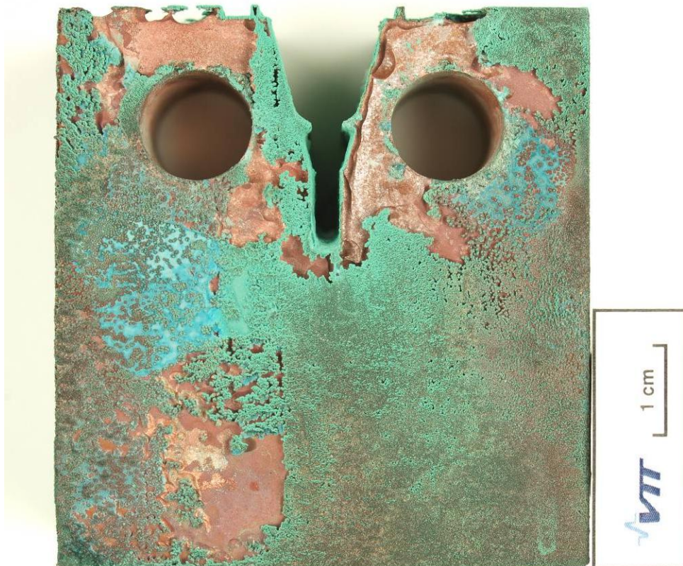
Fig. 8. Extensive general corrosion in the CT specimen after 4400 h (90°C) in aerated simulated Olkiluoto groundwater
