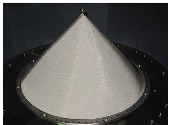
Fig. 2. The heater and thermocouple arrangement and the test bed filled with particles for the COOLOCE-1 and COOLOCE-2 experiments. The diameter of the cone is 500 mm.
