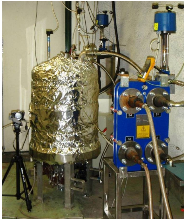
Fig. 1. The COOLOCE pressure vessel (with thermal insulation) and the condenser during the first experiments with conical particle bed.
